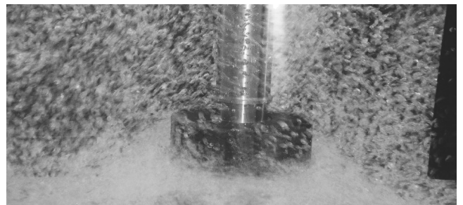
Fig. 9. Gas bubbles generated by the impeller No 1 (350 rpm, 15 dm 3 /min)
