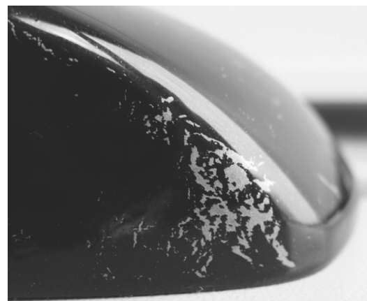
Fig. 3. Disadvantage of paint coating on a car doorknob
