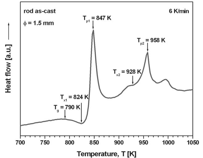
Fig. 4. DSC curve of  $\text{Fe}_{43}\text{Co}_{14}\text{Ni}_{14}\text{B}_{20}\text{Si}_5\text{Nb}_4$  glassy rod with diameter of 1.5 mm
