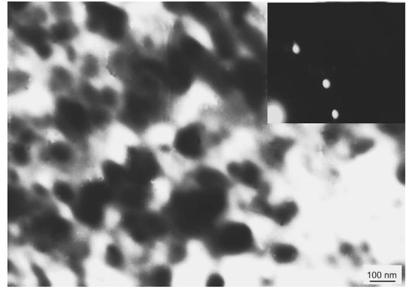
Fig. 6. TEM micrograph plus electron diffraction pattern of Fe<sub>43</sub>Co<sub>14</sub>Ni<sub>14</sub>B<sub>20</sub>Si<sub>5</sub>Nb<sub>4</sub> rod after annealing at 923 K for 1 hour
