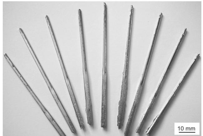
Fig. 1. Outer morphology of glassy  $\text{Fe}_{43}\text{Co}_{14}\text{Ni}_{14}\text{B}_{20}\text{Si}_5\text{Nb}_4$  rods in as-cast state
