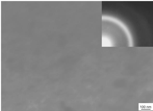
Fig. 3. TEM micrograph plus electron diffraction pattern of  $\text{Fe}_{43}\text{Co}_{14}\text{Ni}_{14}\text{B}_{20}\text{Si}_5\text{Nb}_4$  glassy rod in as-cast state
