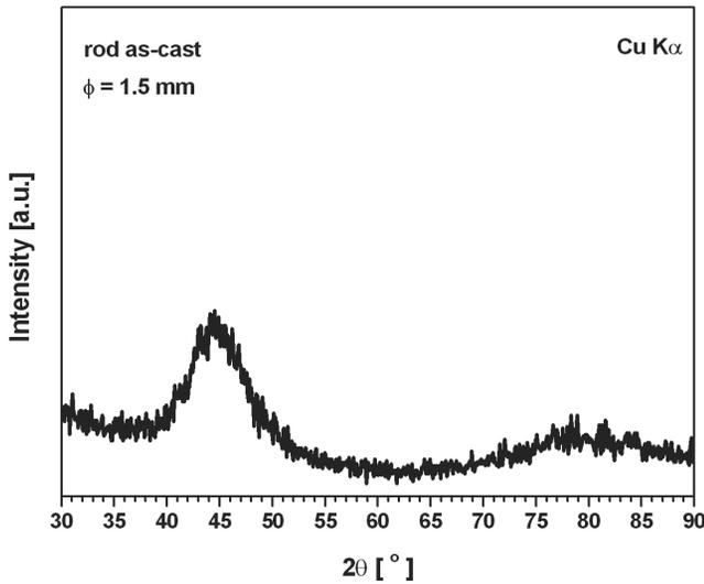
Fig. 2. X-ray diffraction pattern of  $\text{Fe}_{43}\text{Co}_{14}\text{Ni}_{14}\text{B}_{20}\text{Si}_5\text{Nb}_4$  glassy rod in as-cast state
