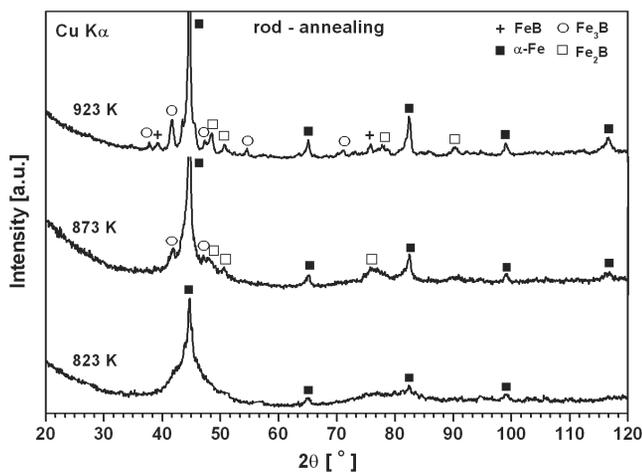
Fig. 5. X-ray diffraction patterns of Fe<sub>43</sub>Co<sub>14</sub>Ni<sub>14</sub>B<sub>20</sub>Si<sub>5</sub>Nb<sub>4</sub> rod after annealing at 823, 873 and 923 K for 1 hour
