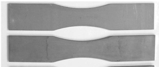
Fig. 2. Traditional fatigue test specimens (steel samples)
