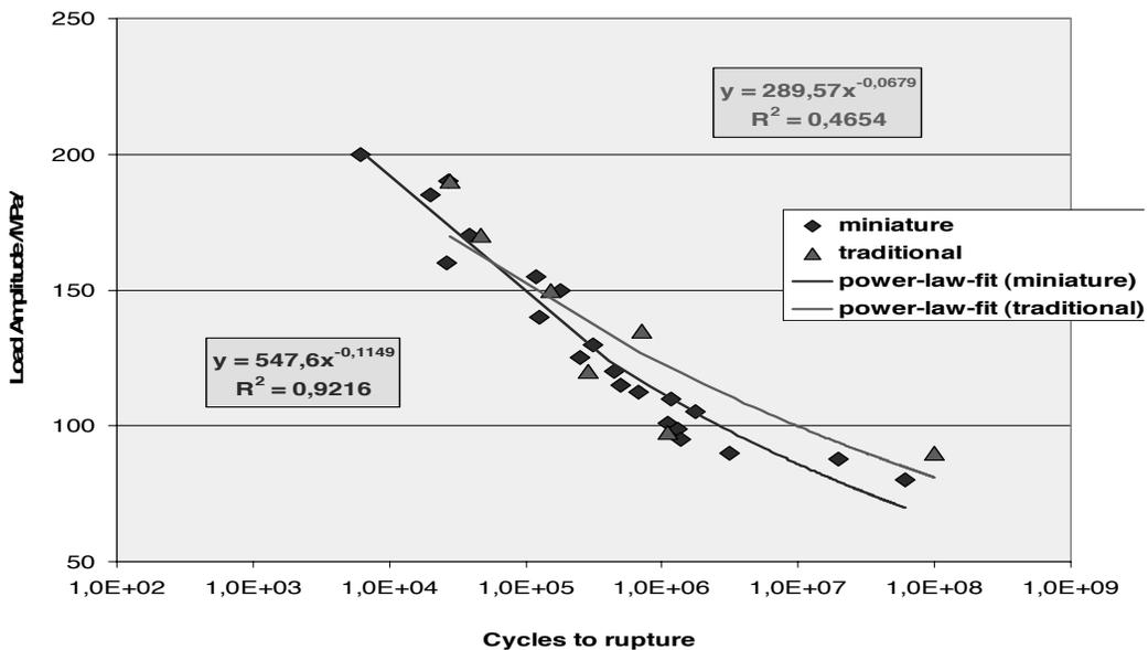
Fig. 10. Comparison of S - N Curves for Al-alloy
