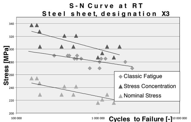
Fig. 6. S-N Curves of the X3 steel
