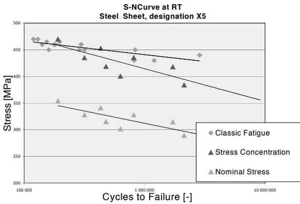
Fig. 7. S-N Curves of the X5 steel
