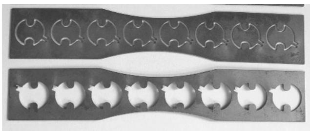
Fig. 3. Miniature fatigue test specimens (steel samples)
