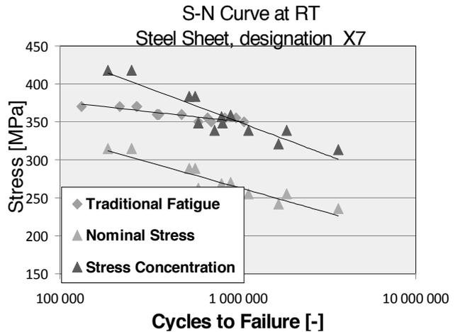
Fig. 9. S-N Curves of the X7 steel
