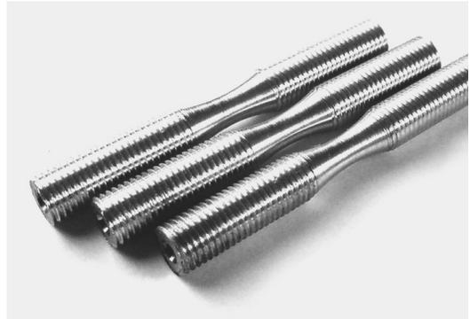
Fig. 4. Traditional fatigue test specimens (Al-alloy)
