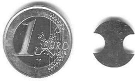
Fig. 1. Miniature fatigue test specimen
