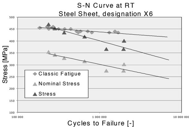
Fig. 8. S-N Curve of the X6 steel
