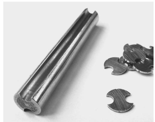
Fig. 5. Miniature fatigue test specimens (Al-alloy)
