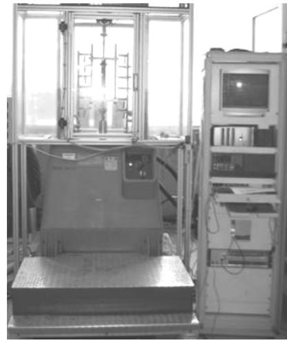
Fig. 1. A servo-hydraulic test-rig used in experimental investigations
