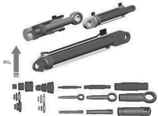
Fig. 7. A modular system of hydraulic cylinders [1]
