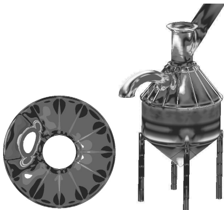
Fig. 13. The von Mises stresses distribution in the dustcatcher (cold-hot scale of values is applied)
