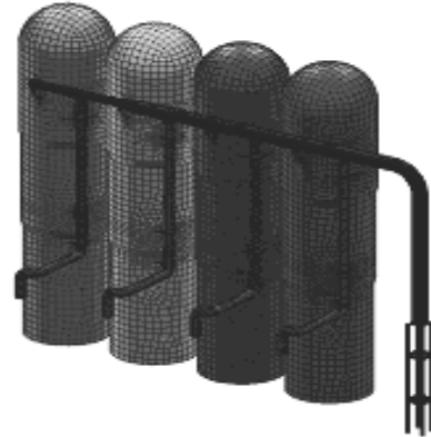
Fig. 9. Hot blast stoves discrete model
