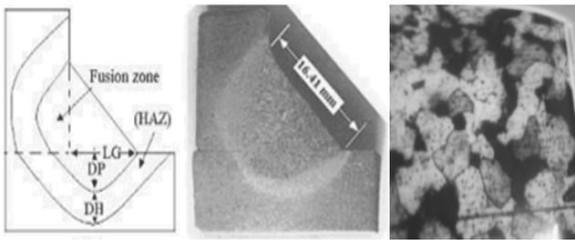
Fig. 3. Different Zones, metallographic photo and the microstructure of Fillet weld
