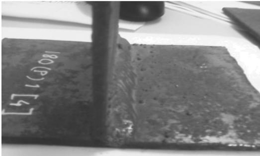
Fig. 2. Schematic Diagram and photo of a one sided fillet joint. The fillet to be modeled is numbered from 22 to 24 in the schematic diagram
