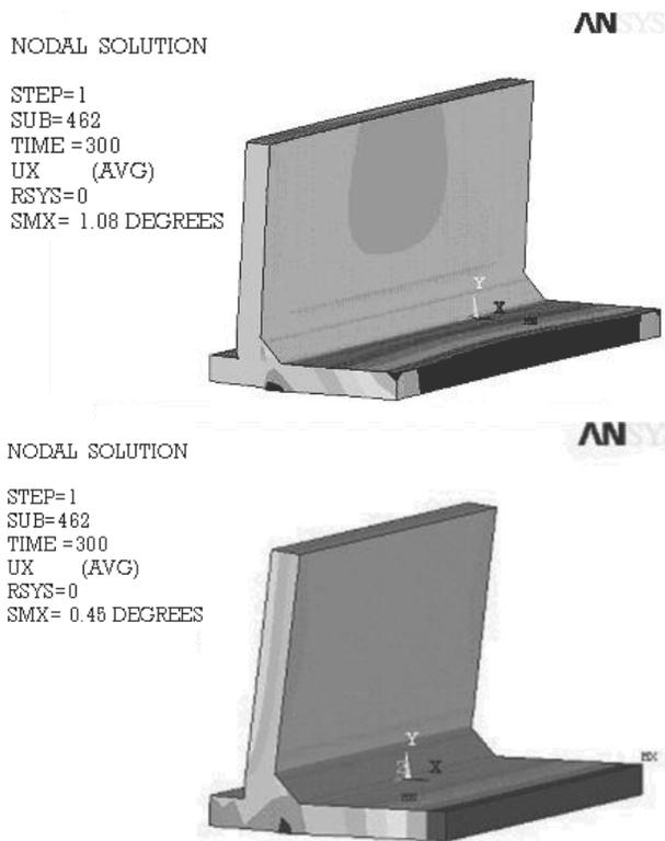
Fig. 4. The deflection of the vertical plate and horizontal plate as obtained by finite element modelling
