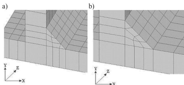
Fig. 1. Modelling and meshing of: (a) 6.5 mm thick one-sided fillet welds (jobs 4 and 5) and (b) 6.5 mm thick one-sided fillet welds (jobs 18 and 19) adopting leg lengths obtained from the experiments
