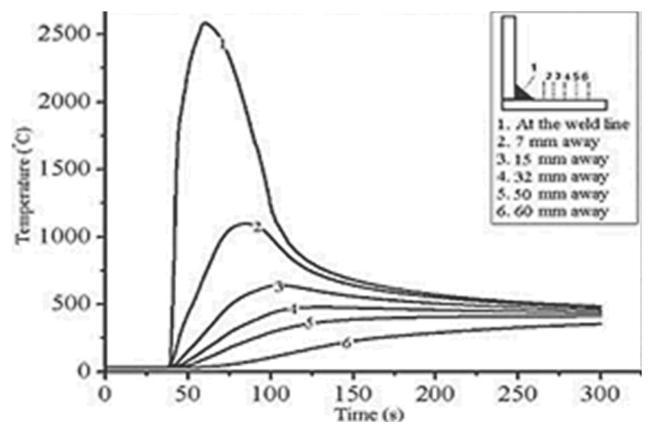
Fig. 5. Predicted surface temperature distribution on the top of the plate
