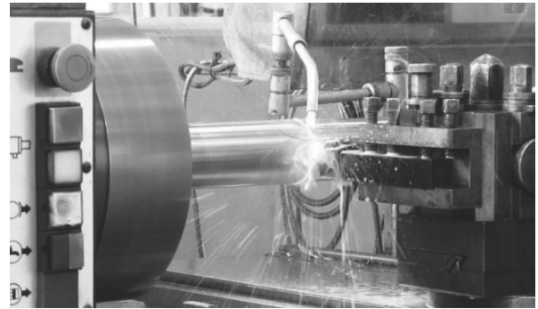
Fig. 8. Burning of chips due to high temperature generation
