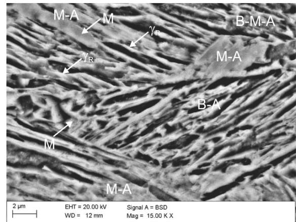
Fig. 7. Microstructure of bainitic ferrite containing interlath retained austenite and martensite-austenite islands of 5MnAlNb
