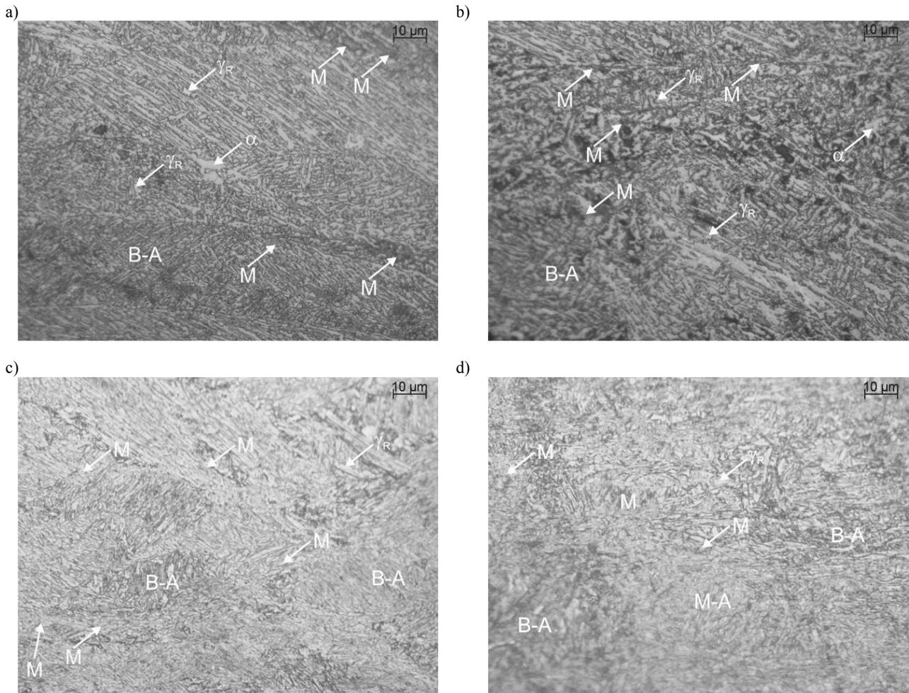
Fig. 5. Bainitic-martensitic-ferritic microstructures of the 3MnAl (a), 3MnAlNb (b) steels and bainitic-martensitic microstructures of the 5MnAl (c), 5MnAlNb (d) steels containing fine granules and interlath retained austenite (after thermomechanical rolling);  $\alpha$  - ferrite,  $\gamma_R$  - retained austenite, M - martensite, B-A - bainitic-austenitic regions, M-A - martensitic-austenitic regions
