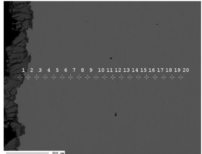
Fig. 4. Schematic of measurement points of chemical composition by WDS from the edge to the middle region of the 3.3 sheet of 5MnAl steel
