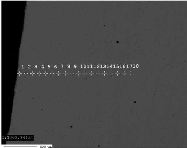
Fig. 3. Schematic of measurement points of chemical composition by WDS from the edge to the middle region of the 3.3 sheet of 3MnAl steel
