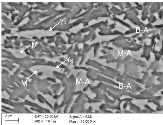
Fig. 6. Microstructure of bainitic ferrite containing interlath retained austenite and martensite-austenite islands of 3MnAlNb
