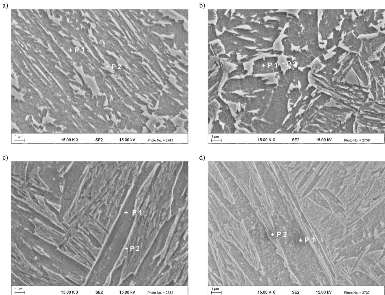
Fig. 2. Bainitic-martensitic microstructures of the 3MnAl (a), 3MnAlNb (b), 5MnAl (c) and 5MnAlNb (d) steels containing cementite and retained austenite of a different morphology depending on the Mn and Nb content (after hot forging)
