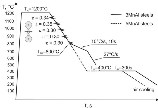
Fig. 1. Thermomechanical rolling schedule of 9 mm steel sheets to a final thickness of 3.3 mm
