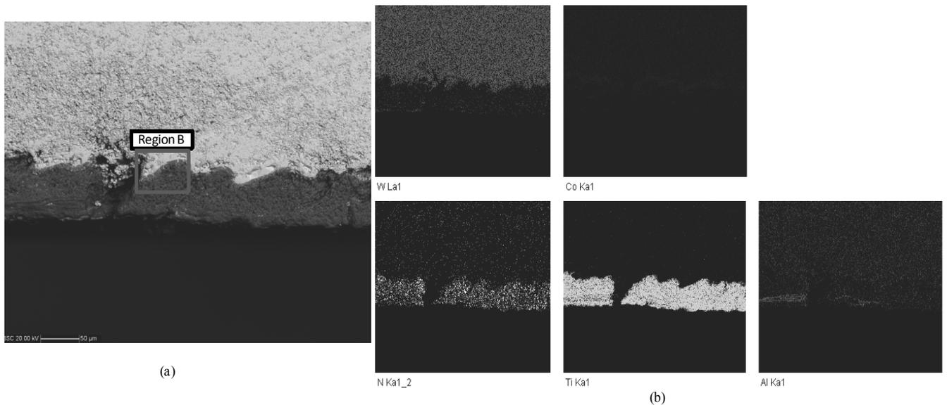
Fig. 10. (a) “Region A” - BSE micrograph showing severe deformation of the WC area, (b) mapping of “Region A” showing materials constituents, especially TiN
