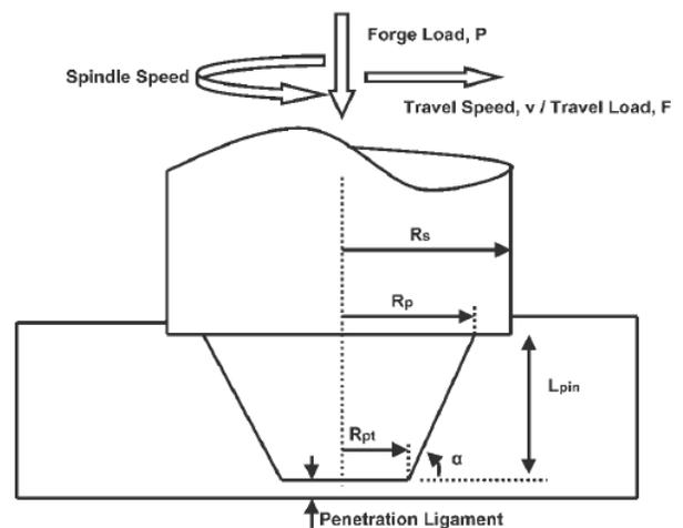
Fig. 3. Basic geometry for FSW tool [5]
