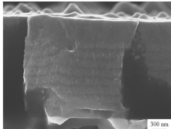
Fig. 2. Micrograph of the (Al, Cr) N coating deposited onto the sintered carbide substrate [7]
