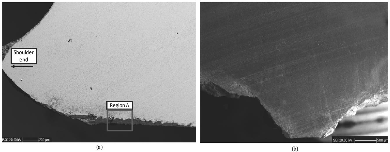
Fig. 9. (a) Transversal micrograph of tool shoulder; (b) transversal micrograph of tool pin showing the fractured region
