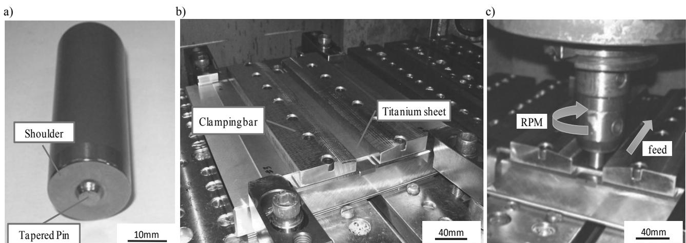
Fig. 5. (a) Tool design showing the pin and shoulder features, (b) fixture device used for the experiment and (c) the tool fixed in the machine spinning and advancing on the titanium sheet
