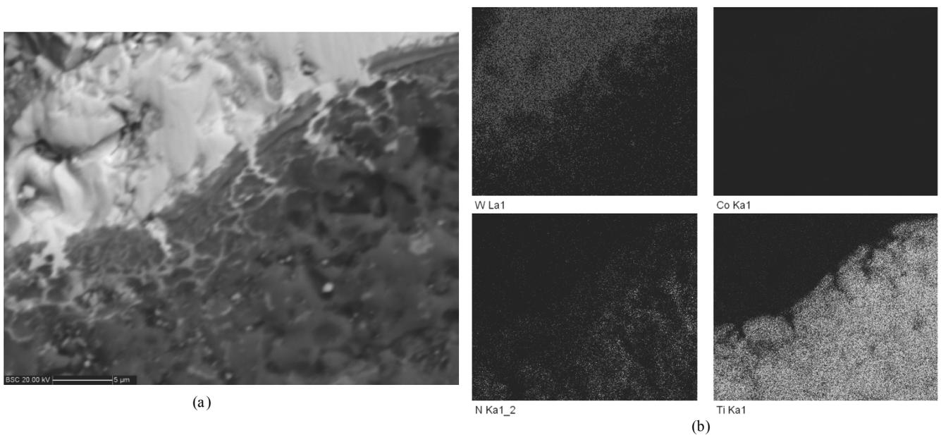
Fig. 11. (a) "Region B" - BSE micrograph showing diffusion mechanism, (b) mapping of "Region B" showing materials interface
