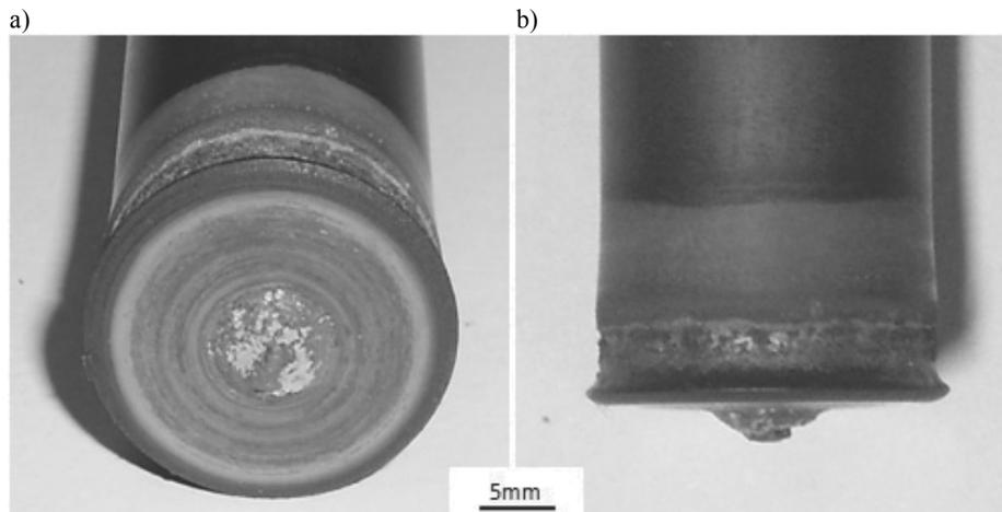
Fig. 6. (a) Front view of the worn tool after the FSW process, (b) side view of the worn tool
