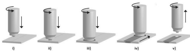
Fig. 1. FSW process steps [3]
