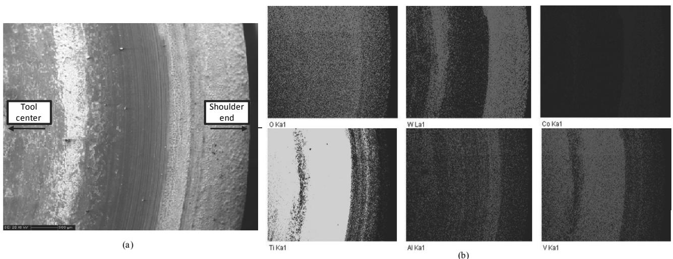
Fig. 8. (a) Micrograph of tool shoulder showing; (b) EDX maps of tool shoulder showing the components found
