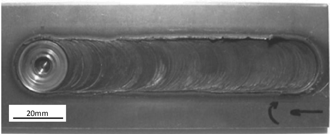
Fig. 4. Aspect of the FSW processed region of the Ti-6Al-4V sheet
