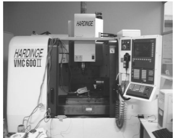
Fig. 2. Experimental Setup for ball end milling of Inconel 718-workpiece
