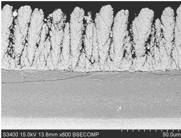
Fig. 2. The microstructure of the ceramic coating obtained by PS-PVD
