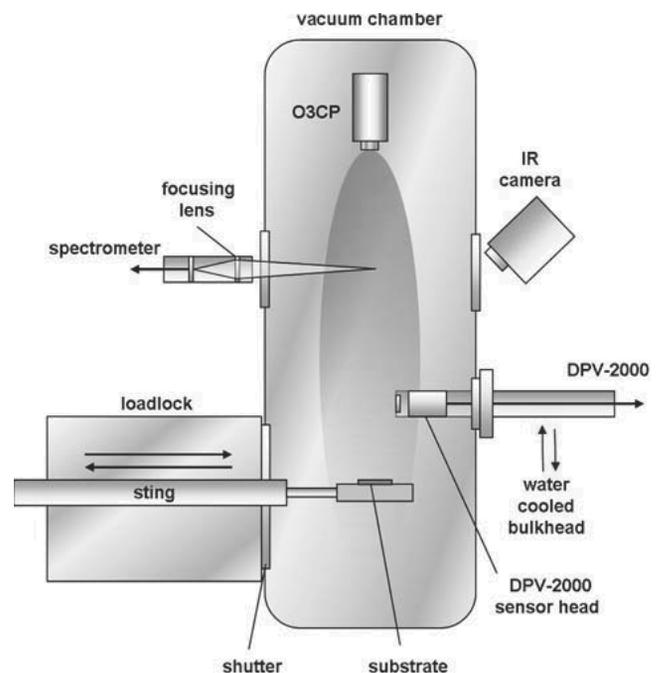
Fig. 3. A diagram of the deposition chamber for the PS-PVD process, showing the placement of monitoring devices (Sulzer-Metco) [10]
