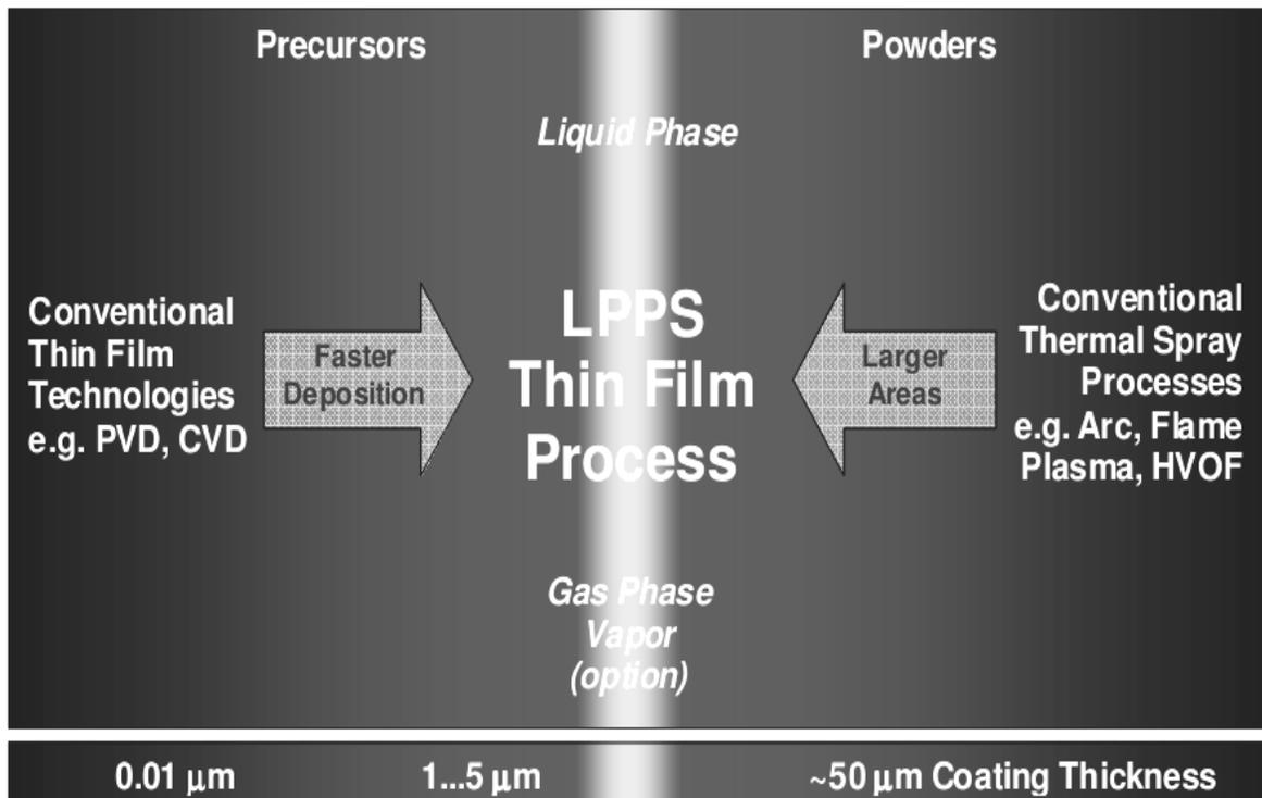
Fig. 1. The distinctive properties of LPPS-Thin Film and PS-PVD processes (Sulzer Metco) [10]
