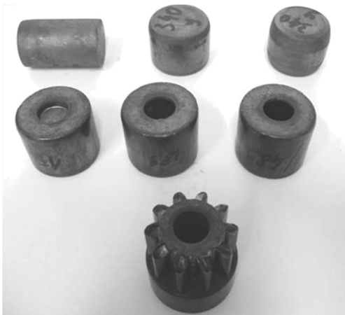
Fig. 3. Three stages of forming for the pinion with chamfered gear
