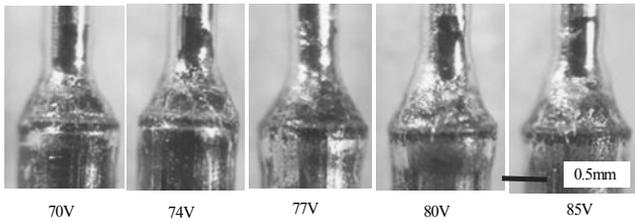
Fig. 7. Change of normal welding shape by welding voltage
