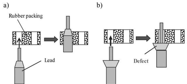
Fig. 10. Effect of welding shape on packing process, a) Normal welded lead, b) Sn-less welded lead
