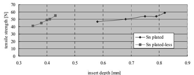
Fig. 14. Tensile strength of vertical direction by insert depth
