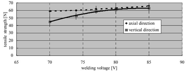
Fig. 19. Tensile strength of Sn-less mold welding by welding voltage
