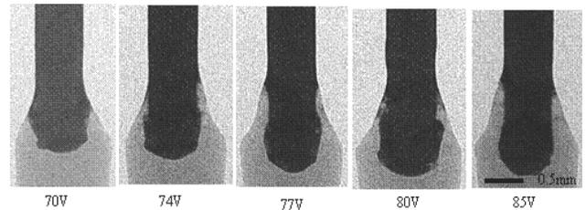
Fig. 12. X-ray photograph of normal welding by welding voltage
