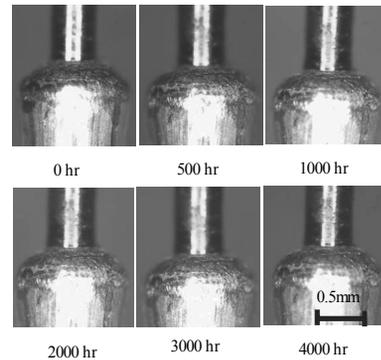
Fig. 26. Whisker accelerated test on 55°C, 85%
