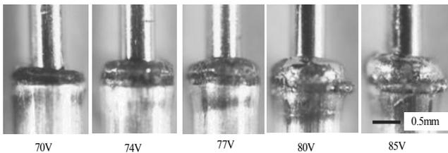
Fig. 17. Change of Sn-less mold welding shape by welding voltage with mold depth 0.6 mm
