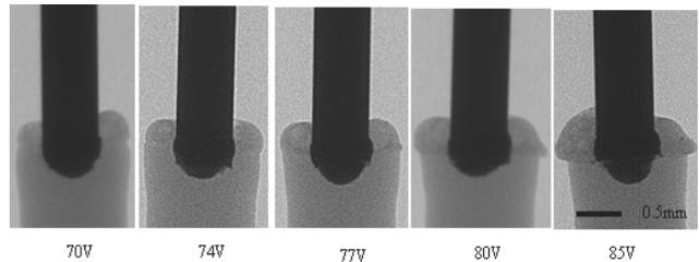
Fig. 21. X-ray photograph of Sn-less mold welding by welding voltage
