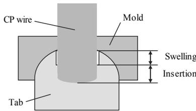
Fig. 23. CP wire supported by swelling and insertion parts
