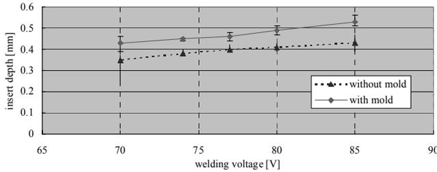
Fig. 22. Insert depth of Sn-less welding by welding voltage
