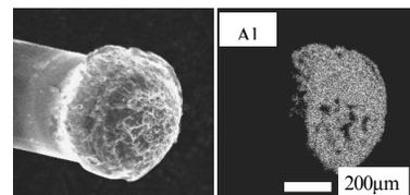
Fig. 15. EDS analysis of CP wire after tensile test with Sn-less CP wire
