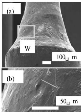
Fig. 2. Whisker at weld point a) weld point, b) detail observation of box region of W
