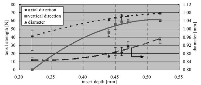
Fig. 25. Tensile strength and diameter of Sn-less mold welding by insert depth
