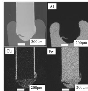
Fig. 20. Cross-sectional EDS analysis of the weld with Sn-less CP wire by mold
