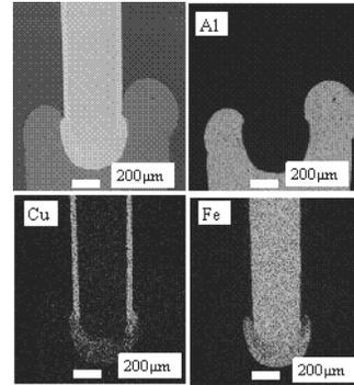
Fig. 9. Cross-sectional EDS analysis of the weld with Sn-less CP wire
