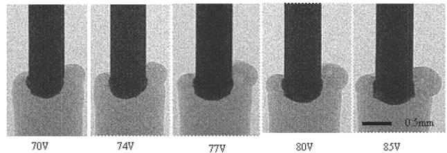
Fig. 13. X-ray photograph of Sn-less welding by welding voltage
