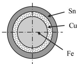
Fig. 3. Schematic structure of Sn and Cu plated Fe wire (named CP wire) structure for aluminum electrolytic condenser
