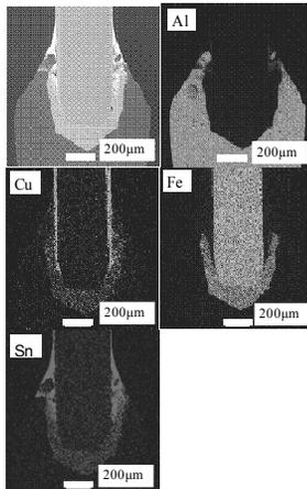
Fig. 6. Cross-sectional EDS analysis of the weld with Sn plated CP wire
