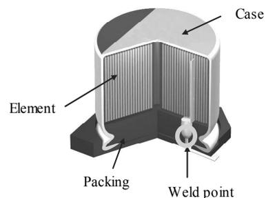
Fig. 1. Detail section structure of aluminum electrolytic condenser and weld point
