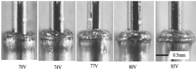
Fig. 16. Change of Sn-less mold welding shape by welding voltage with mold depth 0.3 mm
