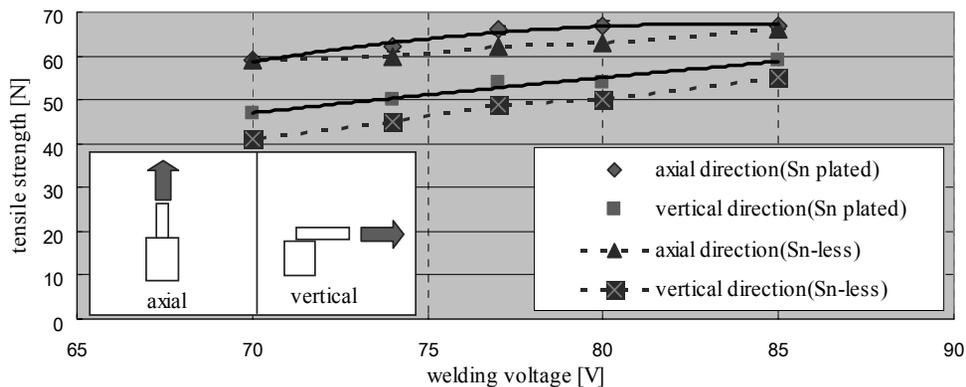
Fig. 11. Tensile strength by welding voltage
