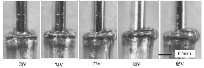
Fig. 8. Change of Sn-less welding shape by welding voltage
