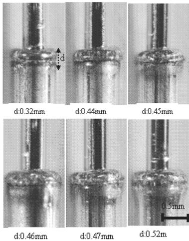
Fig. 24. Change of Sn-less mold welding shape by insert depth(d) at 77V
