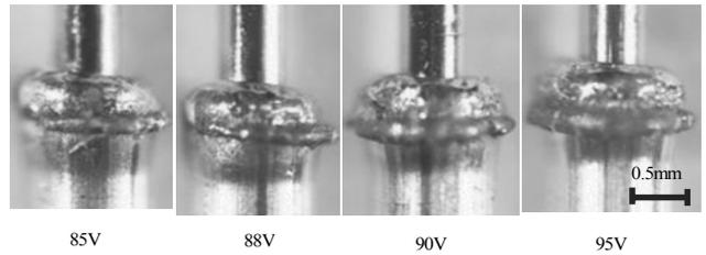
Fig. 18. Sn-less mold welding shape by welding voltage with mold d NG condition
