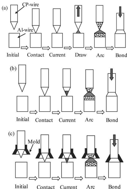
Fig. 4. Percussion welding process with Al-wire and CP-wire
