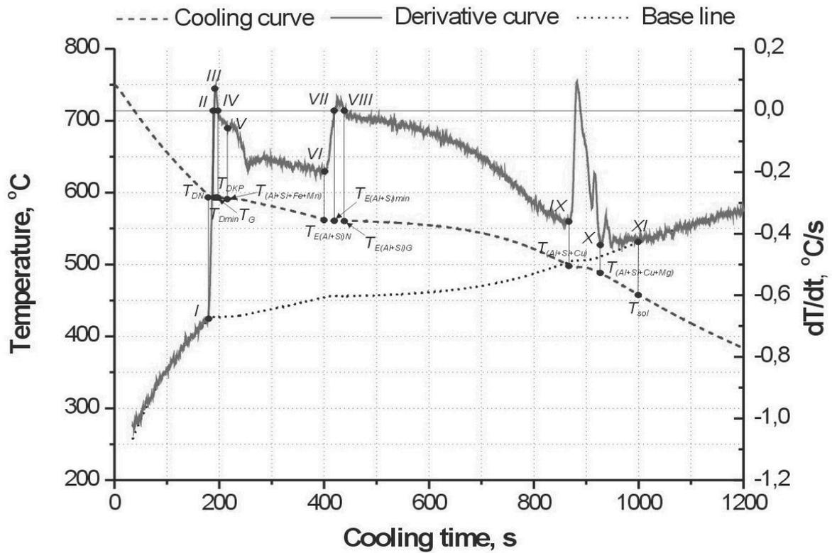
Fig. 9. Cooling and crystallisation curve and the calorimetric analysis of the ATD diagram for the AC AlSi<sub>7</sub>Cu<sub>4</sub> alloy, cooling rate 0.2°C/s
