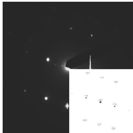
Fig. 8. Diffraction pattern of the Al<sub>2</sub>Cu phase in Fig. 5, zone axis [-621]
