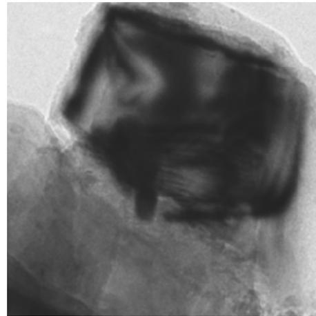
Fig. 6. Al<sub>2</sub>Cu phase in the Al matrix, bright field
