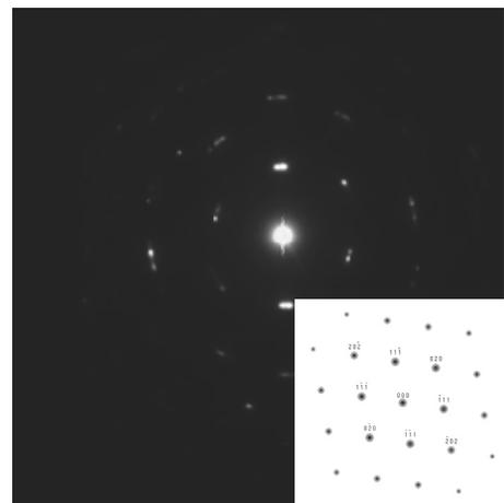
Fig. 4. Diffraction pattern of the Al  $\alpha$  phase in Fig. 2 zone axis, [-10-1]
