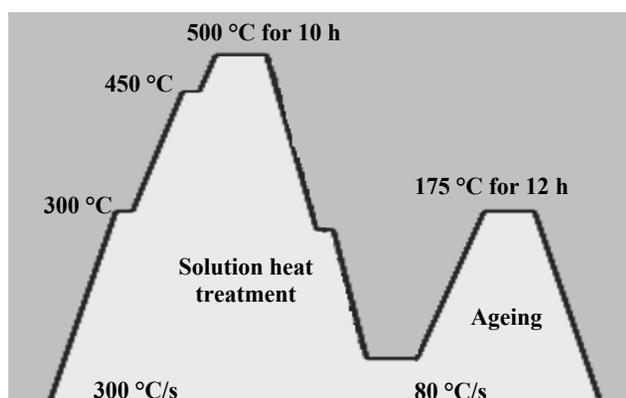
Fig. 2. Heat treatment parameters used for the investigated aluminium cast alloys
