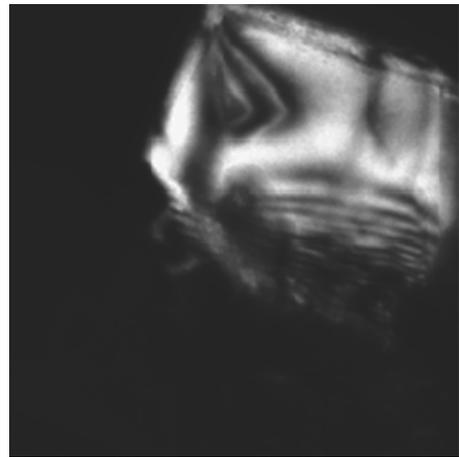
Fig. 7. Al<sub>2</sub>Cu phase in the Al matrix, dark field
