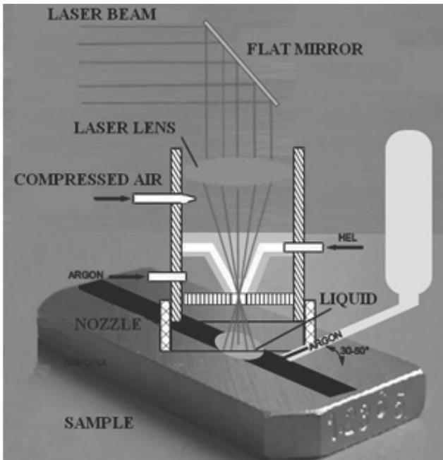
Fig. 1. Scheme of the laser alloying process performed on the investigated AlSi<sub>7</sub>Cu<sub>4</sub> alloy
