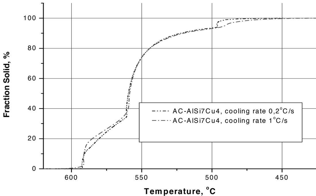
Fig. 10. Fraction solid of the AlSi<sub>7</sub>Cu<sub>4</sub> alloy
