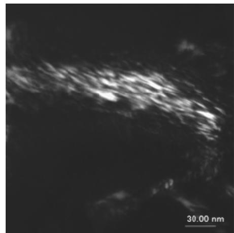
Fig. 5. Structure of the  $\text{Al}\alpha$  phase, dark field
