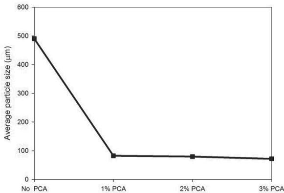
Fig. 8. Laser particle analyser results of 7.5 hr milled aluminium with 0 to 3 wt% of stearic acid
