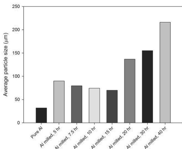
Fig. 6. Laser particle analyser results of pure and milled aluminium in different milling times
