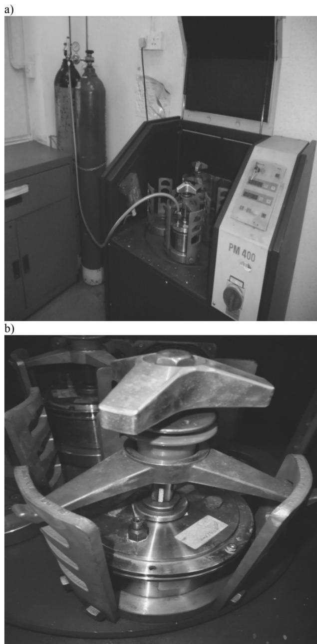
Fig. 1. Retsch PM400 (a), and 500 ml jar single station (b)
