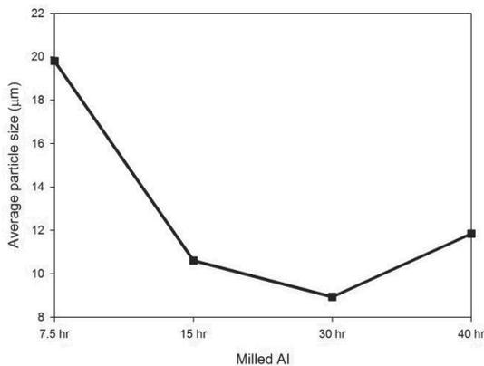
Fig. 13. Laser particle analyser results for 7.5-40 hr milled aluminium with methanol
