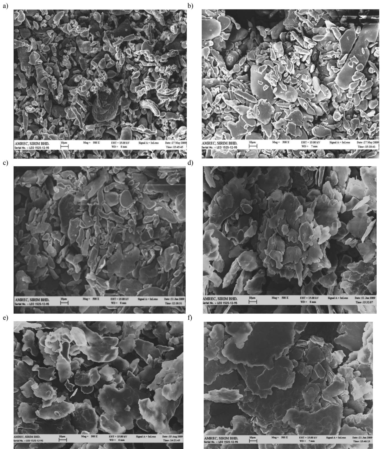
Fig. 5. SEM micrograph for: a) unmilled pure aluminium, b) 5 hr milled aluminium powder, c) 10 hr milled aluminium powder, d) 20 hr milled aluminium powder, e) 30 hr milled aluminium powder, f) 40 hr milled aluminium powder
