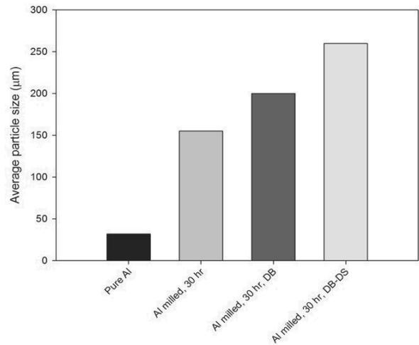
Fig. 10. Laser particle analyser results of 30 hr milled aluminium with different ball size (10, 15 and 20 mm), ball no. (31) and rotation speed (250 rpm)
