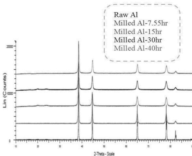
Fig. 3. X-Ray diffraction (XRD) pattern of unmilled and milled aluminium powder
