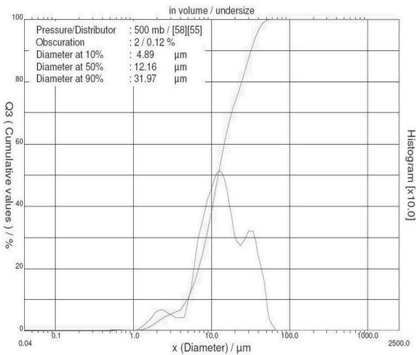
Fig. 2. Particle analyser graph (CILAS 11900) of pure aluminium
