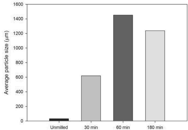
Fig. 4. Laser particle analyser for unmilled and 0.5-3 hr milled aluminium without argon and PCA
