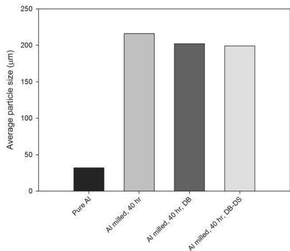
Fig. 11. Laser particle analyser results for pure aluminium and 40 hr milled Al with different ball sizes (10, 15 and 20 mm), ball no. (31) and rotation speed of 250 rpm.
