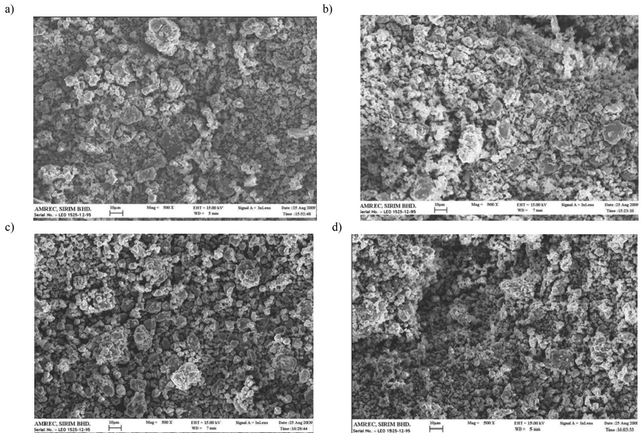
Fig. 12. SEM micrograph of: 7 hr (a), 15 hr (b), 30 hr (c) and 40 hr (d) milled aluminium with methanol
