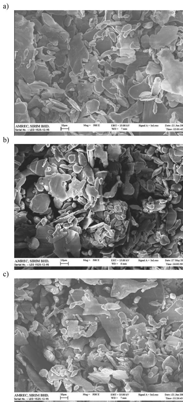
Fig. 7. SEM micrograph of 7.5 hr milled aluminium with: a) 1 wt% of stearic acid, b) 2 wt% of stearic acid, c) 3 wt% of stearic acid
