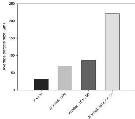
Fig. 9. Laser particle analyser results of 15 hr milled Al with different ball size (10, 15, 20 mm), ball no. (31) and rotation speed (250 rpm)
