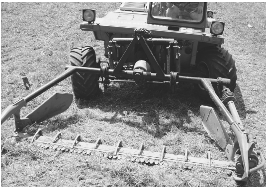
Fig. 4. A double blade mower REFORM applied in our experiment
