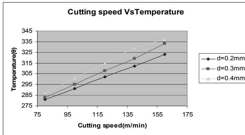
Fig. 9. Cutting Speed Vs Temperature for different Depth of cut
