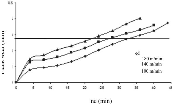
Fig. 3. Flank Wear Vs Machining time for different cutting speeds (Tool: Alumina, Work: AISI 304)
