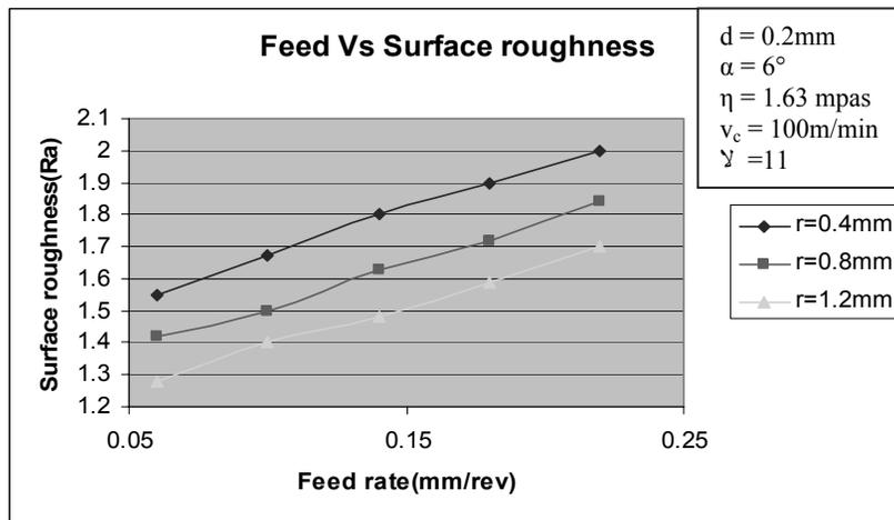
Fig. 6. Feed rate Vs Surface roughness for different Nose radius
