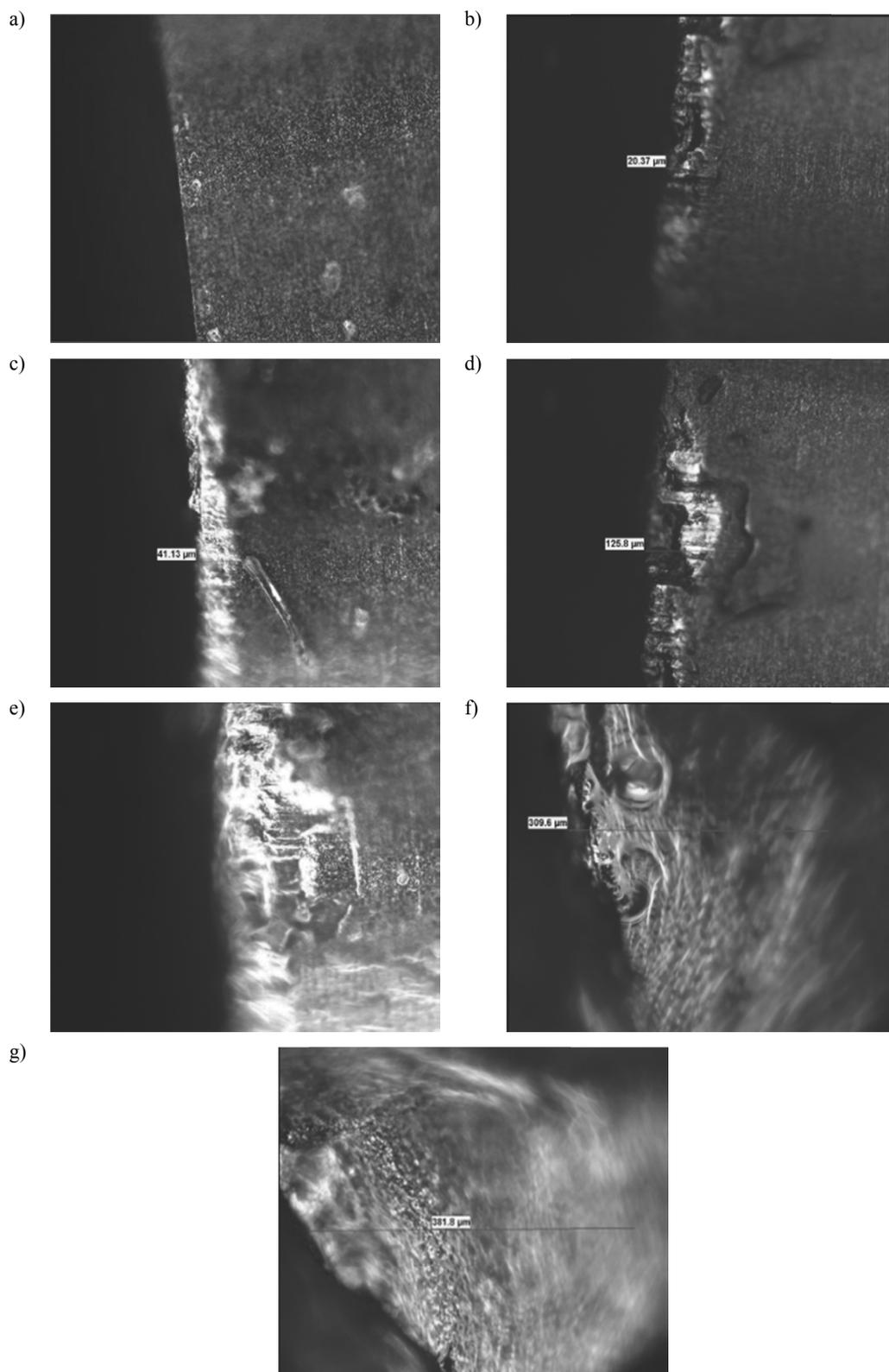
Fig. 4. Flank Wear propagation in alumina inserts at interval of 6 minutes
