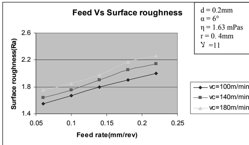
Fig. 5. Feed rate Vs Surface roughness for different Cutting speed
