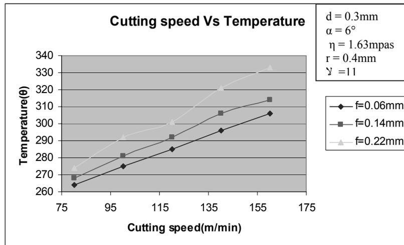
Fig. 8. Cutting Speed Vs Temperature for different Feed rates
