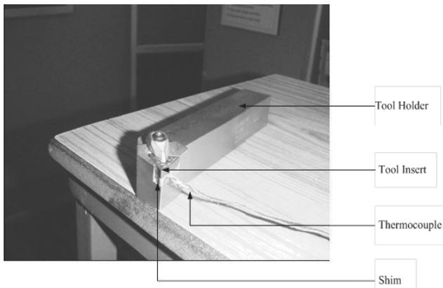
Fig. 2. Cutting zone temperature measuring system
