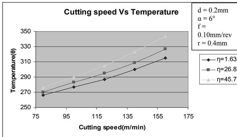
Fig. 7. Cutting Speed Vs Temperature for different Cutting fluid
