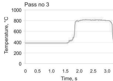
Fig. 7. Temperature values registered on a surface of 5Mn-A steel sheet after the third pass by a stationary pyrometer
