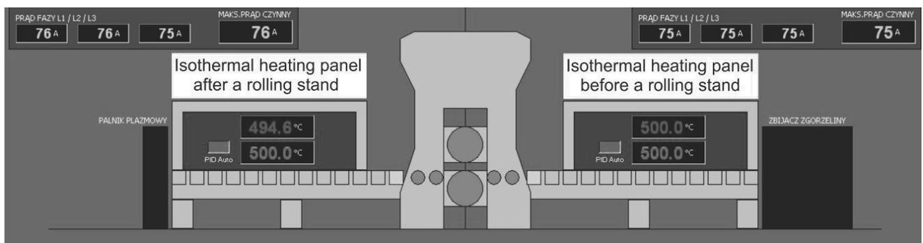
Fig. 2. Schematic of isothermal heating panels before and after a rolling stand
