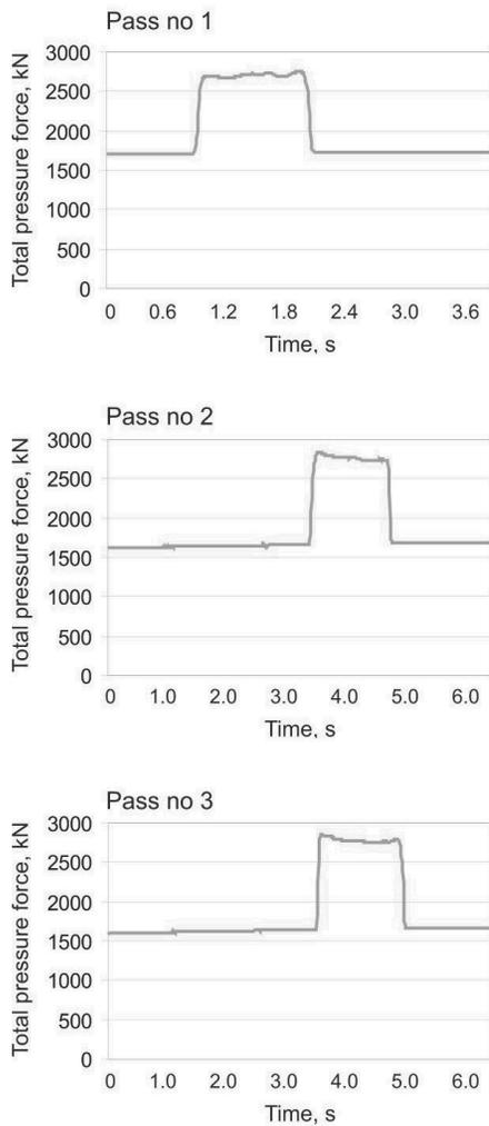
Fig. 6. Registration of the total pressure force for the 5Mn-A steel strip hot-rolled in three passes
