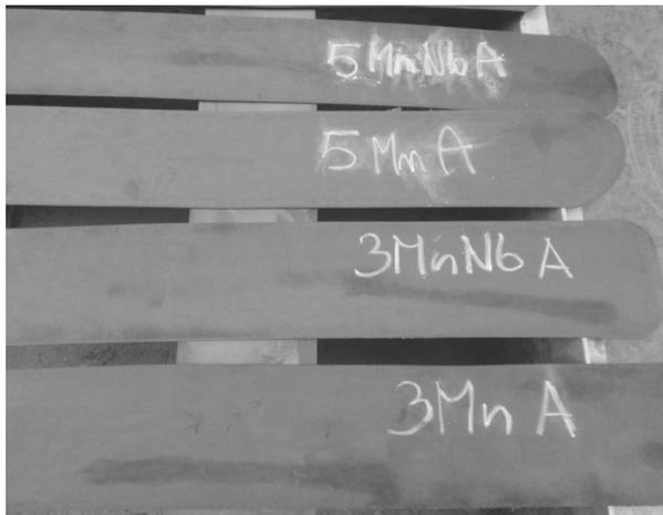
Fig. 5. Strips of 4.5 mm thickness thermomechanically rolled in 3 passes
