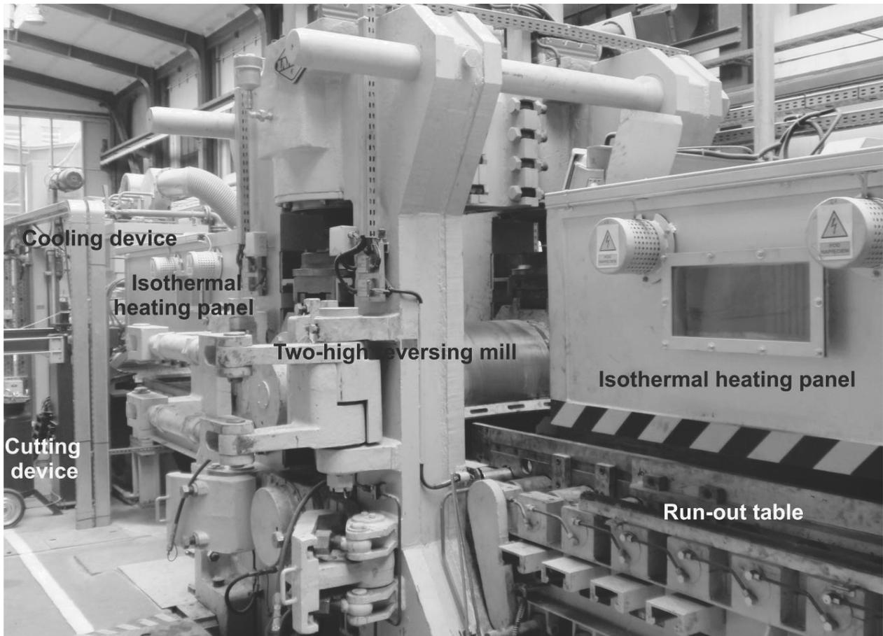
Fig. 1. Semi-industrial line for simulation of hot rolling and controlled cooling of sheets and bars at the Institute for Ferrous Metallurgy in Gliwice, Poland
