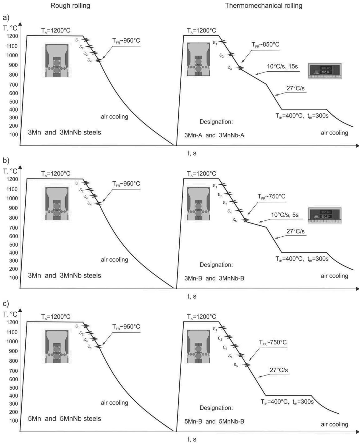
Fig. 4. Rough rolling paths and subsequent thermomechanical processing schedules designed for hot rolling of 9 mm thick steel sheets in 3 passes (a) and in 5 passes (b, c) for 3Mn and 3MnNb steels (a, b) and 5Mn and 5MnNb steels (c)
