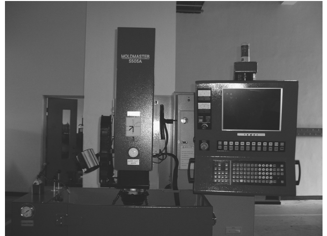
Fig. 1. Photograph of electrical discharge machine used in experimental trials
