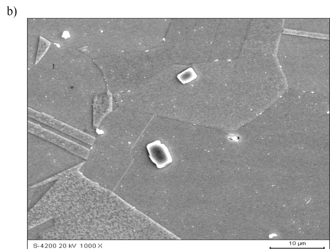
Fig. 6. Microstructure of material of steam superheater coils of T321H austenitic steel in as-received state (test piece no. 10) observed with a) light microscope, b) SEM
