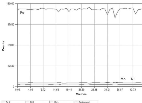
Fig. 6. Distribution of alloying elements: Ni and Mo made EDS analysis for 37MnNiMo6-4-3 hypoeutectoid steel.  $T_A = 850^\circ\text{C}$ ; cooling rate = 1°C/s
