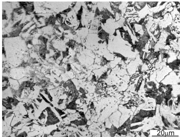
Fig. 4. Microstructures of the 37MnNiMo6-4-3 hypoeutectoid steel after dilatometric test. Etched with 3% nital
