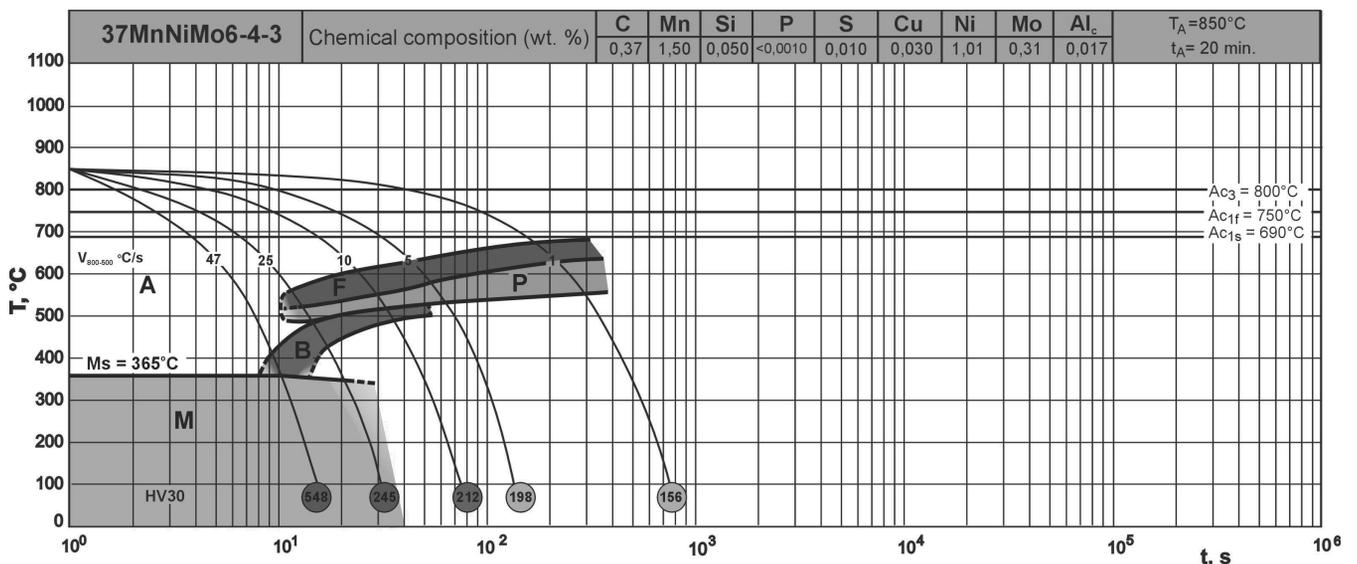
Fig. 3. The CCT diagram of 37MnNiMo6-4-3 steel
