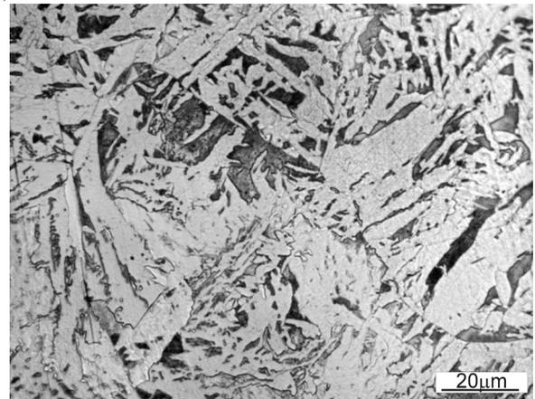
Fig. 1. Microstructure of the 37MnNiMo6-4-3 steel after re forging. Etched by 3% nital
