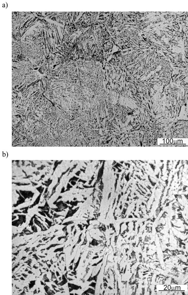
Fig. 2. Microstructure of 37MnNiMo6-4-3 after full annealing. Etched with 3% natal
