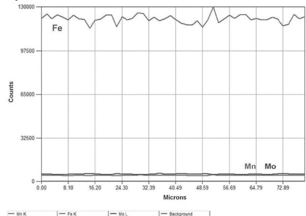
Fig. 5. Distribution of alloying elements: Mn, Ni and Mo made EDS analysis for 37MnNiMo6-4-3 hypoeutectoid steel.  $T_A = 850^\circ\text{C}$ ; cooling rate =  $50^\circ\text{C/s}$
