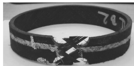
Fig. 9. Image of sample after tensile test NOL ( A=35 MPa, T=30^\circ\text{C} , N=4180 )
