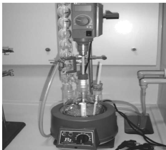
Fig. 3. The laboratory reactor used for the transesterification process
