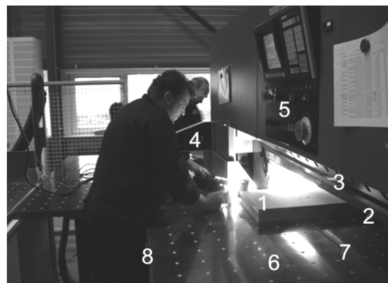
Fig. 4. Front view of guillotine during testing in industrial conditions [8]; 1 - bundle, 2 - pressure beam, 3 - cutting blade with knife holder, 4 - safety curtain, 5 - control, 6 - pneumatic table, 7 - cutting stick, 8 - manual mode push buttons
