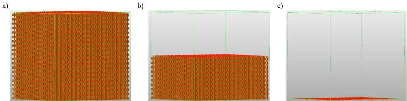
Fig. 5. Example layering one of the designed models. The height of the model is 10 mm, number of layers created is 200, thickness 50 microns: a) 200 layers, b) 100 layers, c) 1 layer
