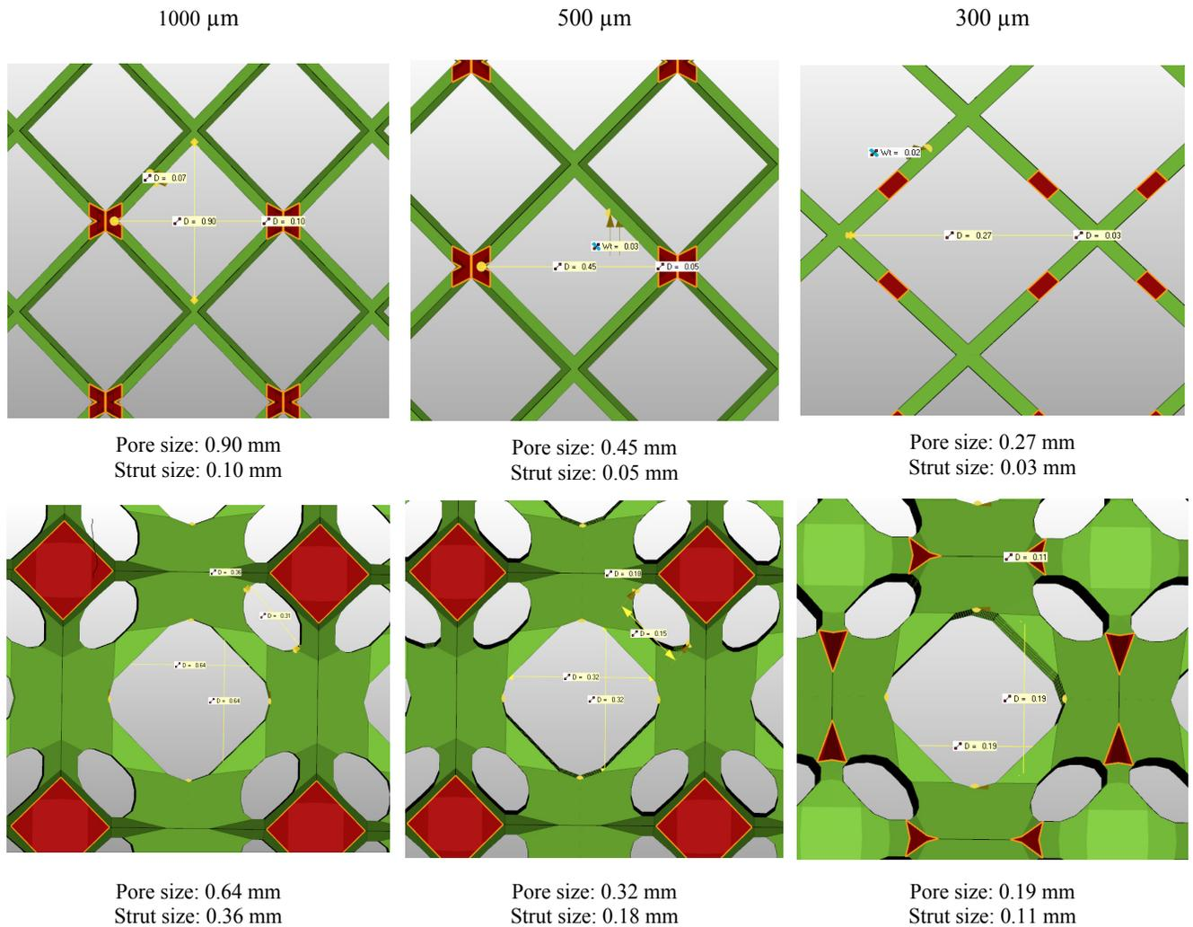
Fig. 9. Measuring the pore size and strut size of the resulting models of the unit cell Fig. 8 a and Fig. 8 b
