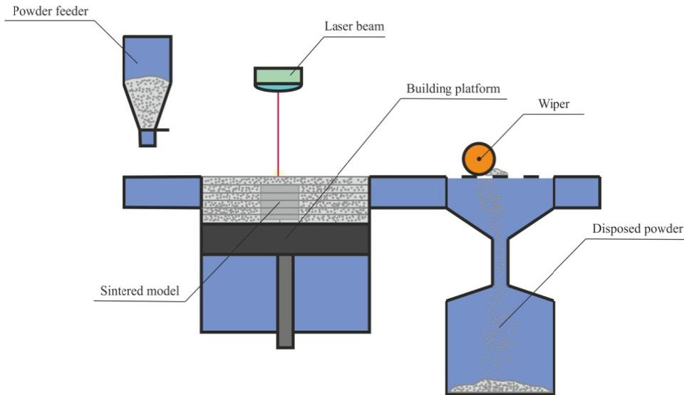
Fig. 2. Scheme of selective laser sintering technique
