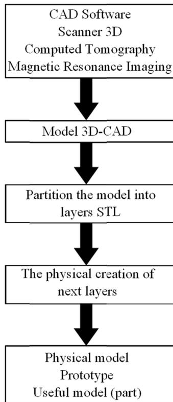
Fig. 1. A schematic outline of additive manufacturing (AM) technology [8]
