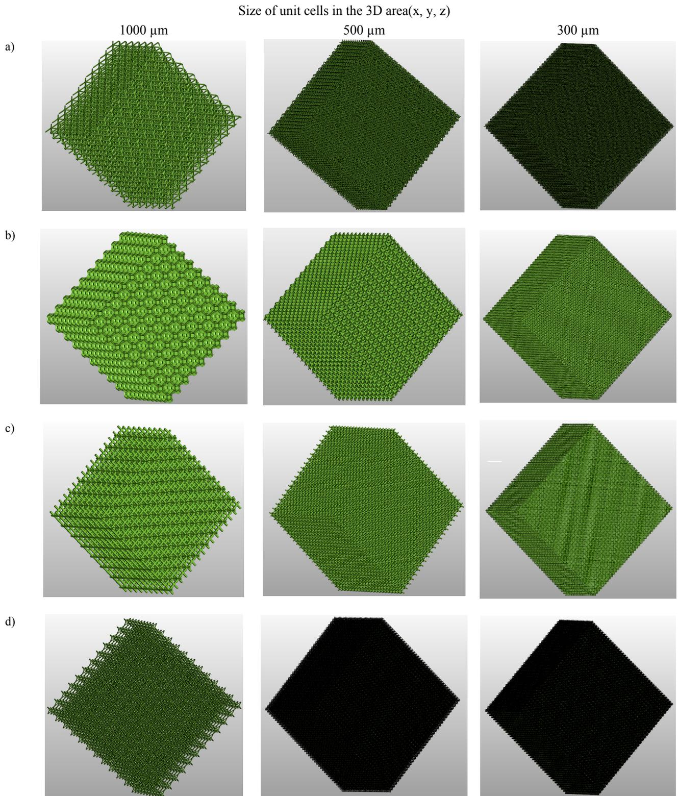
Fig. 7. Models designed in AutoFab software (10x10x10 mm). Pictures shown designed models made of unit cells (according to Fig. 6 a, b, c, d) of different shape and size in the x, y, z
