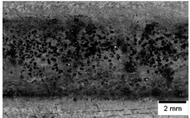
Fig. 14. Surface structure after feeding of the powder \text{ZrO}_2 into the surface layer of the AlSi9Cu, laser power 2.0 kW, 8.0 g/min, scan rate 0.25 m/min
