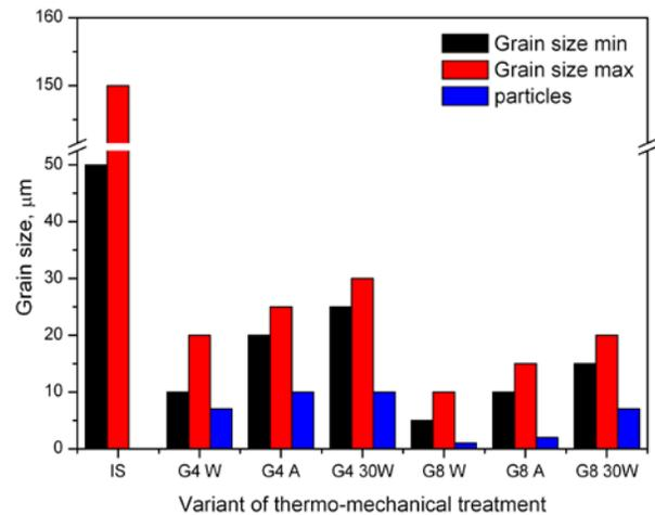
Fig. 8. The grain size of the austenitic steels after different variants of thermo-mechanical deformations carried out on the simulator Gleeble
