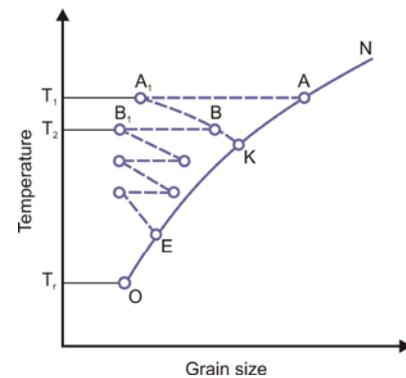
Fig. 1. Influence of temperature and deformation on grain size during multi-stage rolling [12]
