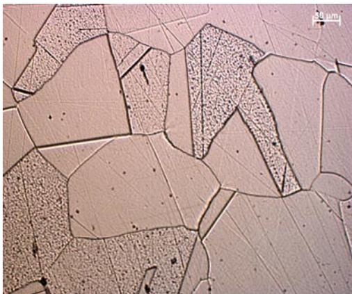
Fig. 5. Steel X11MnSiAl17-1-3 in a initial state
