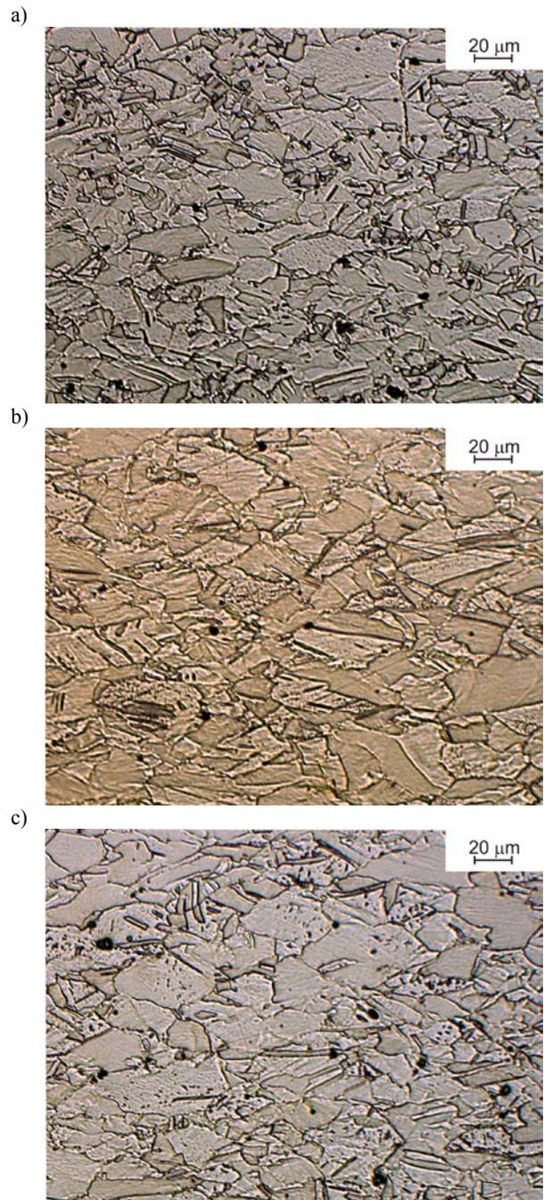
Fig. 6. Structures of high-manganese austenitic X11MnSiAl17-1-3 steel after thermo-mechanical treatment in Gleeble simulator according to schedule shown in Fig. 2 and variant of cooling a) G4W, b) G4A, c) G4 30W
