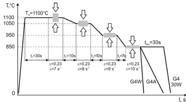
Fig. 2. Schematic and parameters of the 4-stage compression test carried out on Gleeble 3800 thermo-mechanical simulator.  $T_A$  - austenitizing temperature,  $t_{iso}$  - time of the isothermal holding of specimens at temperature of last deformation - 850°C
