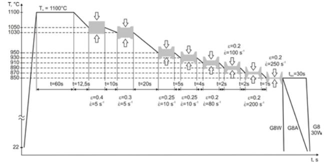
Fig. 3. Schematic and parameters of the 8-stage compression test carried out on Gleeble 3800 thermo-mechanical simulator.  $T_A$  - austenitizing temperature,  $t_{iso}$  - time of the isothermal holding of specimens at temperature of last deformation - 850°C
