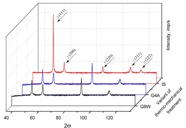
Fig. 4. Comparison of X-ray diffraction pattern after different stages and variants of thermo-mechanical treatment
