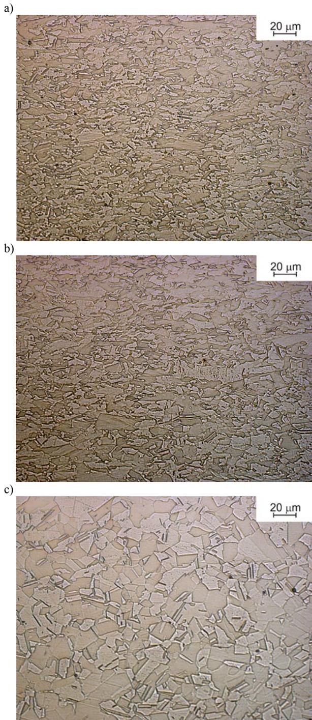
Fig. 7. Structures of high-manganese austenitic X11MnSiAl17-3-1 steel after thermo-mechanical treatment in Gleeble simulator according to schedule shown in Fig. 3 and variant of cooling a) G8W, b) G8A, c) G8 30W
