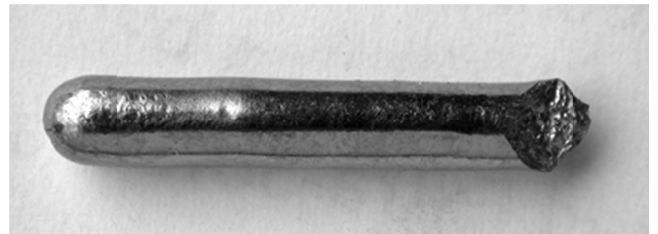
Fig. 5. Macroscopic picture of that sample titanium alloy Ti - 6Al - 4V produced by injection casting
