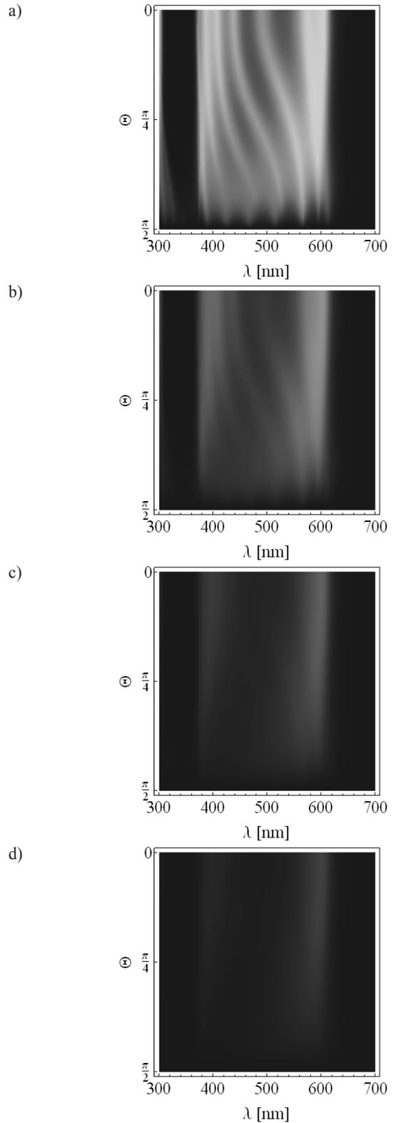
Fig. 3. Binary superlattice unpolarized transmission map for  $L = 7$ ; a)  $k = 0.01$ , b)  $k = 0.03$ , c)  $k = 0.05$ , d)  $k = 0.07$
