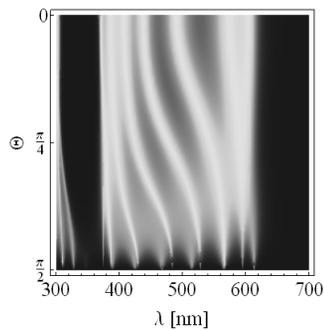
Fig. 2. Binary superlattice unpolarized transmission map for  $L = 7$  and  $k = 0$
