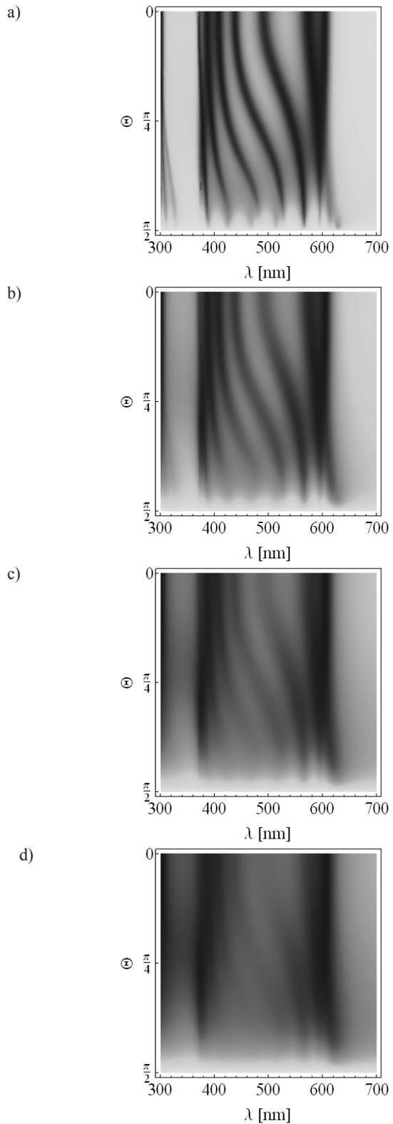
Fig. 6. Binary superlattice unpolarized reflectance map for  $L = 7$ ; a)  $k = 0.01$ , b)  $k = 0.03$ , c)  $k = 0.05$ , d)  $k = 0.07$
