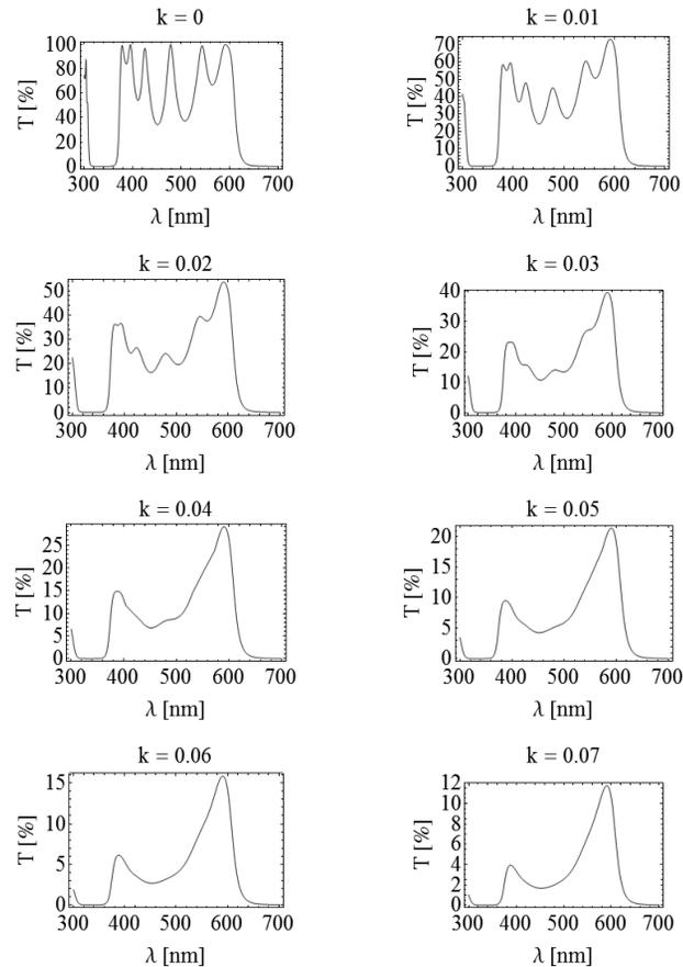
Fig. 4. The transmission of binary structure for the angle of incidence equal to  $\Theta = \pi/4$  and different rates of extinction coefficient  $k$
