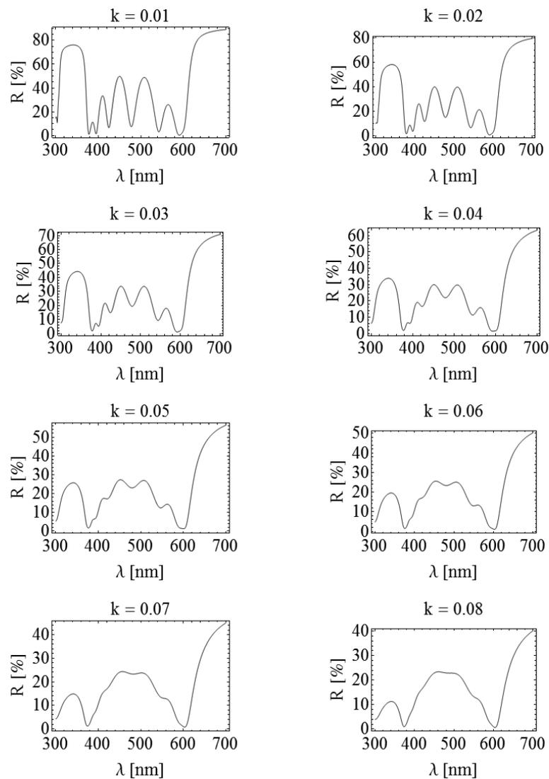
Fig. 7. The reflectance of binary structure for the angle of incidence equal to  $\Theta = \pi/4$  and different rates of extinction coefficient  $k$
