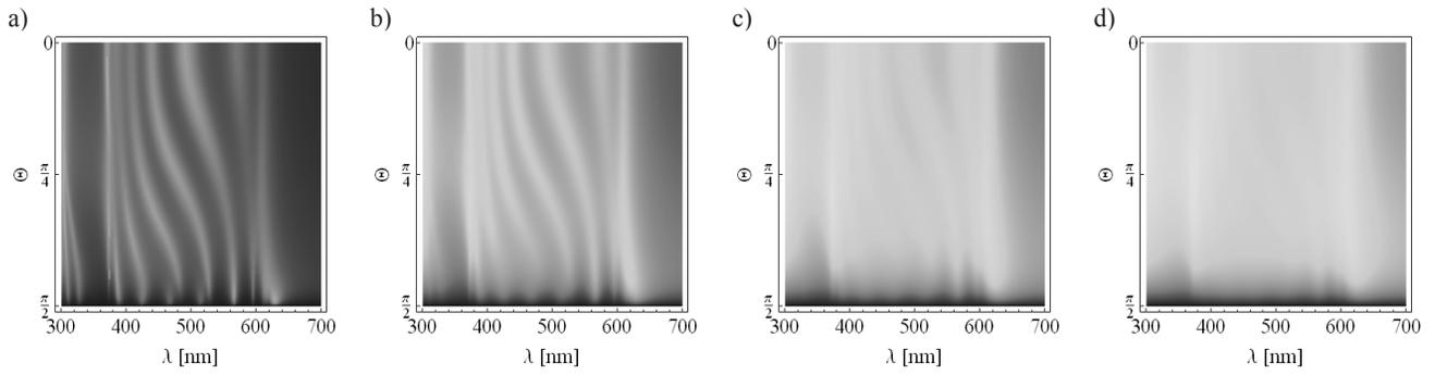
Fig. 9. Binary superlattice unpolarized absorption map for  $L = 7$ ; a)  $k = 0.01$ , b)  $k = 0.03$ , c)  $k = 0.05$ , d)  $k = 0.07$
