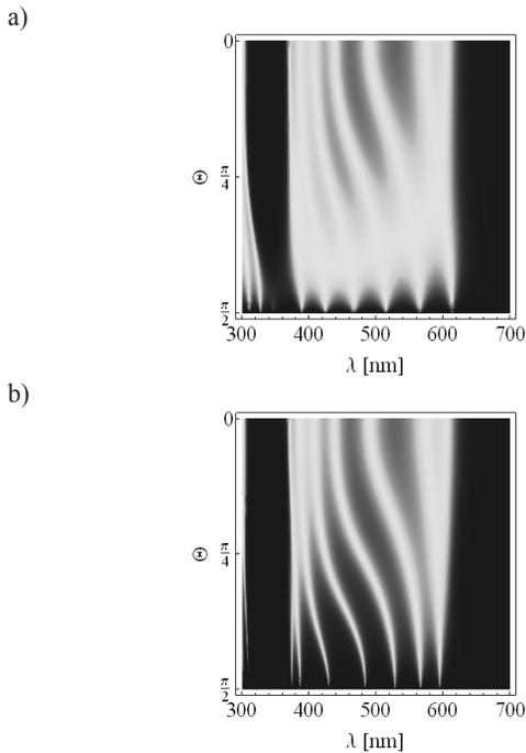
Fig. 1. Binary superlattice transmission map for  $L = 7$ ,  $k = 0$ , a) polarization P, b) polarization S
