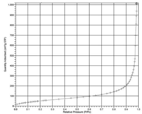
Fig. 7. Isotherm linear plot for Aerosil R812
