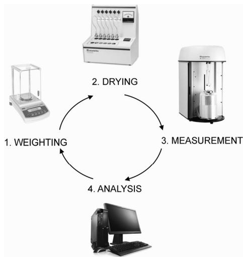
Fig. 2. The circle shows the sequence of steps taken in surface research using gas adsorption method
