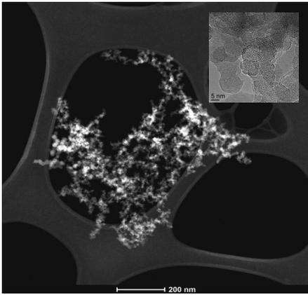
Fig. 3. HAADF STEM image of typical Aerosil DT4 aggregate
