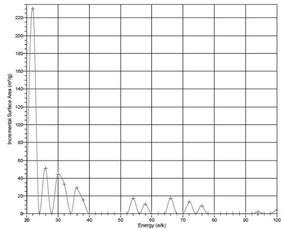
Fig. 15. Incremental Surface Area vs. Energy for Aerosil R812
