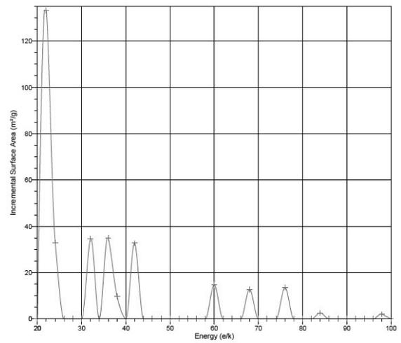
Fig. 14. Incremental Surface Area vs. Energy for Aerosil DT-4
