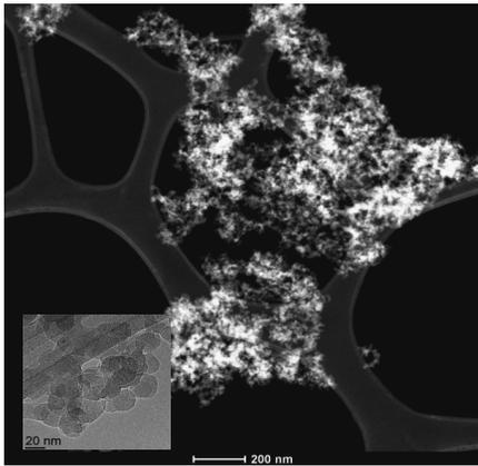
Fig. 4. HAADF STEM image of typical R812 aggregate
