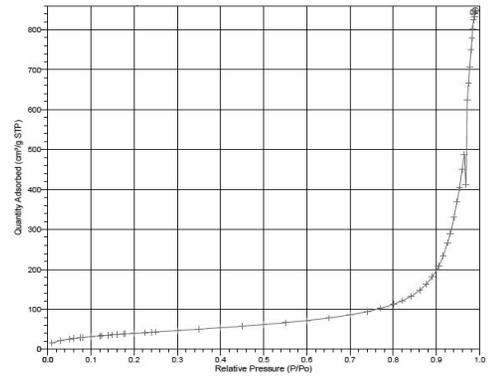
Fig. 6. Isotherm linear plot for Aerosil dt-4
