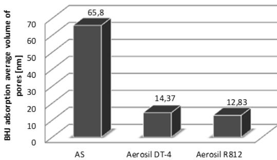
Fig. 12. BHJ adsorption average volume of pores
