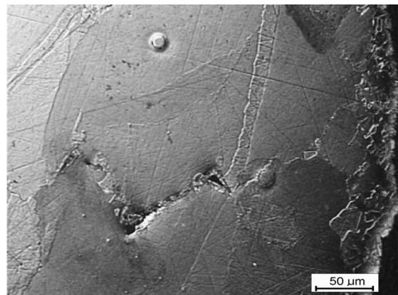
Fig. 9. The structure of CuNi25 alloy sample after deformation at temperature 600°C
