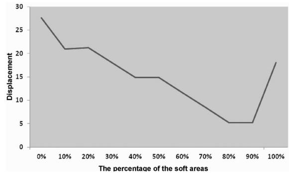
Fig. 5. The results of FEM simulations, displacement of virtual sample versus percentage of the soft areas
