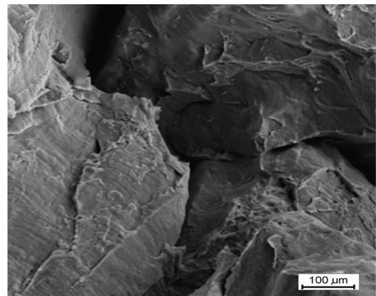
Fig. 10. The fracture of CuNi25 alloy sample after deformation at temperature 525°C (SEM)
