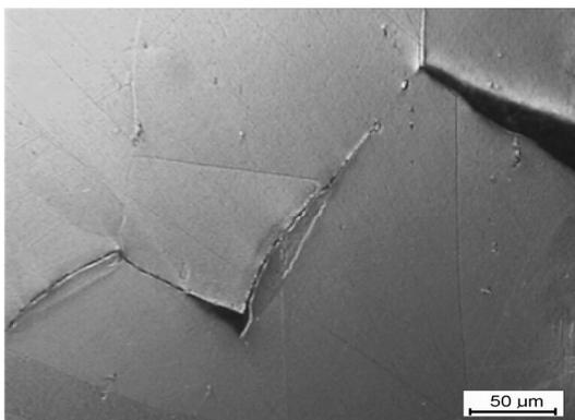
Fig. 8. The structure of CuNi25 alloy sample after deformation at temperature 500°C
