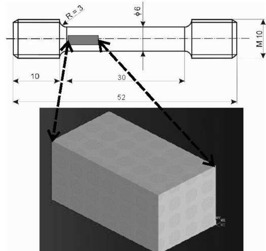
Fig. 2. The real sample and the model of virtual polycrystalline sample of material with "hard core" and "soft mantle" areas used for FEM simulation, based on Kelvin's 14-hadrons
