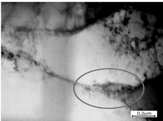
Fig. 7. The structure of CuNi25 alloy sample after deformation at 475°C (TEM)
