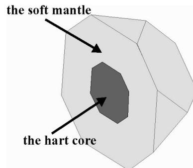
Fig. 3. Model of virtual grain with a hard core and soft mantle shell in single 14-hadron used for FEM simulation
