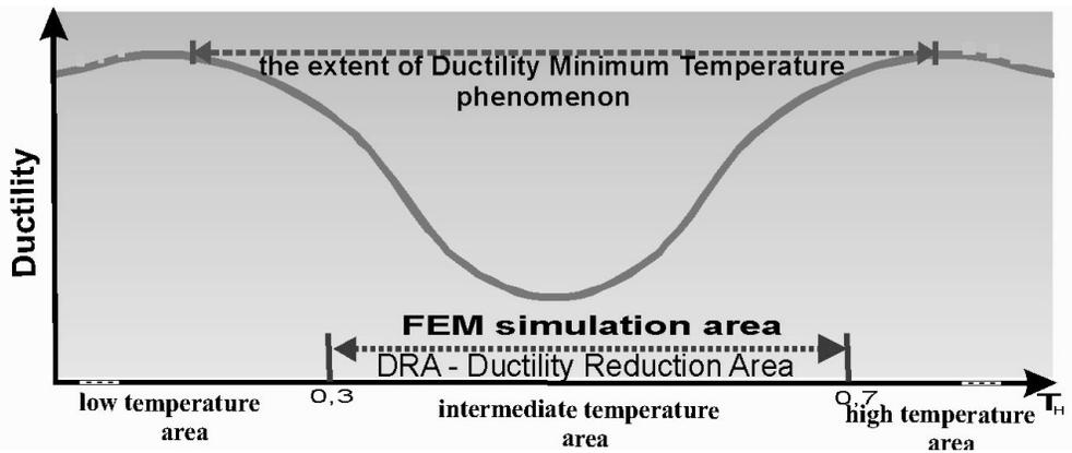
Fig. 1. The range of Ductility Minimum Temperature phenomenon occurrence
