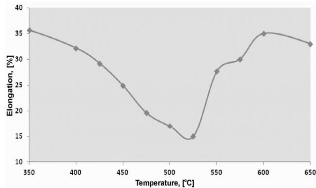
Fig. 4. Elongation versus test temperature for CuNi25, after deformation during high temperature tensile tests with strain rate  $4.2 \cdot 10^{-3} \cdot s^{-1}$
