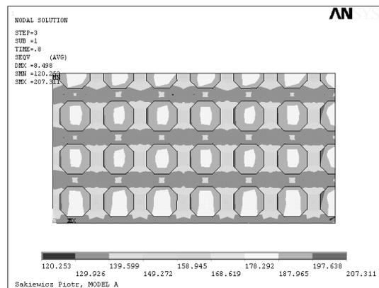
Fig. 6. Stress distribution in the model of 70% of soft areas in the volume of the virtual sample
