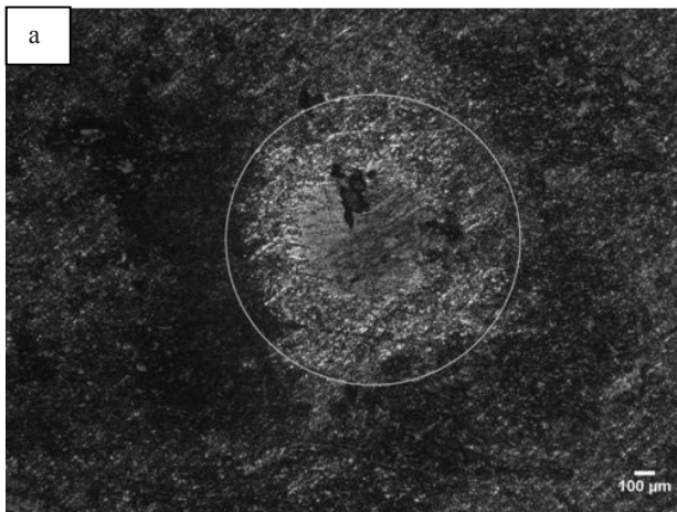
Fig. 12. Microscope figures were obtained after 2h of testing on ball-tester, a) conventional method, b) injection method
