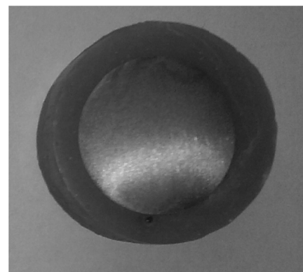
Fig.2. Macroscopic samples of Ti-6Al-4V alloy produced by conventional method
