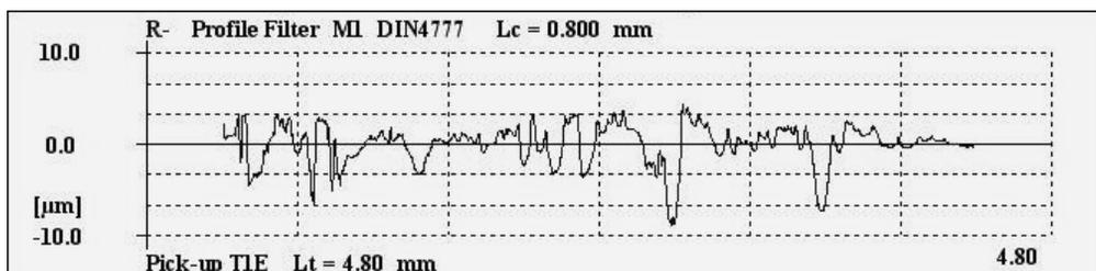
Fig. 7. Third measurement of the abrasion profile for the  $\text{Fe}_{61}\text{Co}_{10}\text{W}_2\text{Y}_2\text{B}_{20}$  sample in plate form
