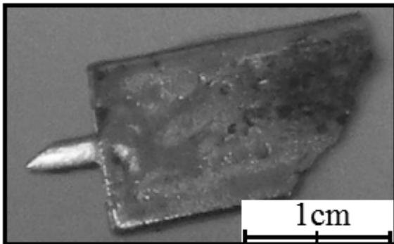
Fig. 1. Example image of the  $\text{Fe}_{61}\text{Co}_{10}\text{W}_2\text{Y}_2\text{B}_{20}$  alloy sample, in the form of a plate, obtained by the injection-casting method
