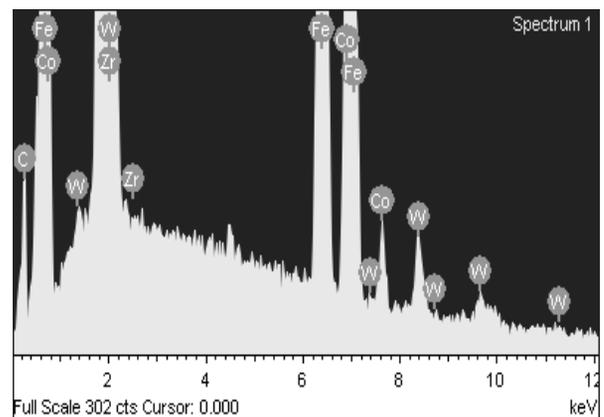
Fig. 3. Spectrum of the chemical elements present on the surface of the investigated sample
