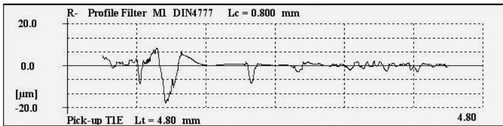
Fig. 5. First measurement of the abrasion profile for the  $\text{Fe}_{61}\text{Co}_{10}\text{W}_2\text{Y}_2\text{B}_{20}$  sample in plate form
