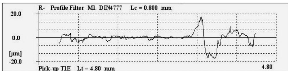
Fig. 8. Fourth measurement of the abrasion profile for the  $\text{Fe}_{61}\text{Co}_{10}\text{W}_2\text{Y}_2\text{B}_{20}$  sample in plate form
