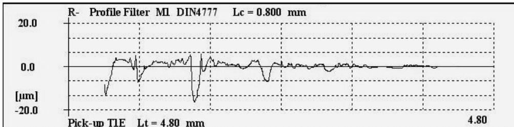
Fig. 6. Second measurement of the abrasion profile for the  $\text{Fe}_{61}\text{Co}_{10}\text{W}_2\text{Y}_2\text{B}_{20}$  sample in plate form
