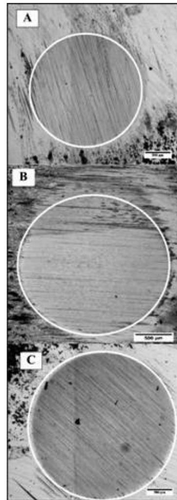
Fig. 4. Images of the abrasion areas, obtained with the magnification of 50x. Time of test: A - 1 hour, B - 2 hours, C - 3 hours
