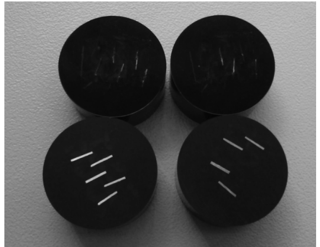
Fig. 1. Samples after mounting, partially sanded and polished
