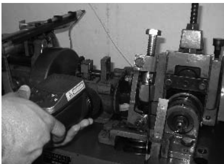
Fig. 10. The temperature recording by infrared camera FLIR ThermoCAM type E
