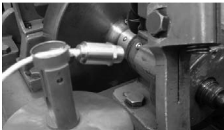
Fig. 5. Application of temperature sensor on tribometer
