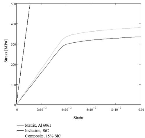
Fig. 3. Stress-strain curves of matrix material, inclusion material and composite material
