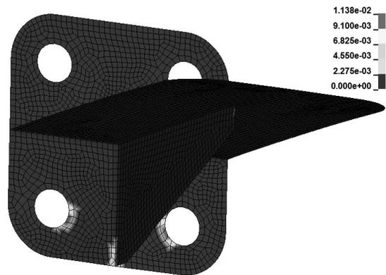
Fig. 14. Accumulated plastic strain in aluminium alloy part, maximum value equals  $1.138 \cdot 10^{-2}$
