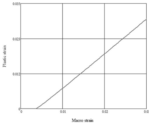
Fig. 6. Plastic strain of matrix phase in function of macro strain in uniaxial state of stress
