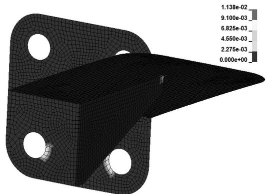
Fig. 13. Accumulated plastic strain in matrix phase of composite cantilever, maximum value equals  $8.232 \cdot 10^{-3}$
