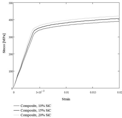
Fig. 4. Estimated stress-strain curves of composites with different volume fraction of reinforcement
