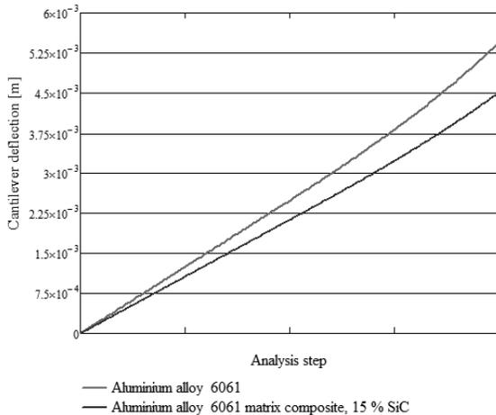
Fig. 15. Deflection comparison of cantilever made of aluminium alloy and cantilever made of aluminium matrix composite
