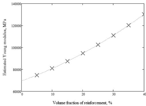
Fig. 5. Composite's Young modulus in function of volume fraction of SiC particles
