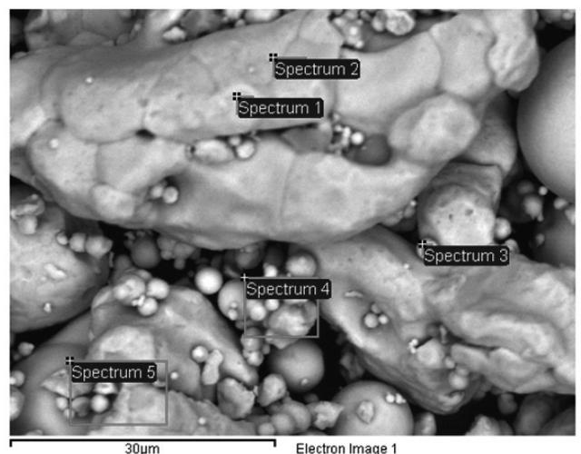
Fig. 6. SEM picture of DSH20 powder before sintering
