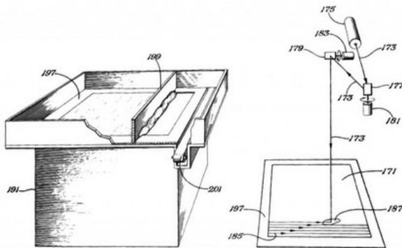
Fig. 1. Schematic diagram of powder sintering method introduced by R.F. Housholder [1]
