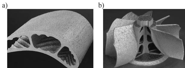
Fig. 2. Aerospace elements manufactured by SLM technology: a - turbine blade for PW4000 HTP engine, b - blade integrated disk (image source: Fraunhofer ILT, Aachen)
