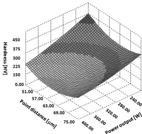
Fig. 14. Hardness vs Point distance and Laser Power with constant exposure time and scan speed (ET = 100  $\mu$ s, SP = 100 mm/s)
