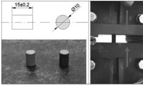
Fig. 9. Samples for measurement of compression strength
