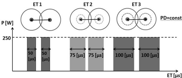
Fig. 7b. Schematic illustration of Exposure Time parameter
