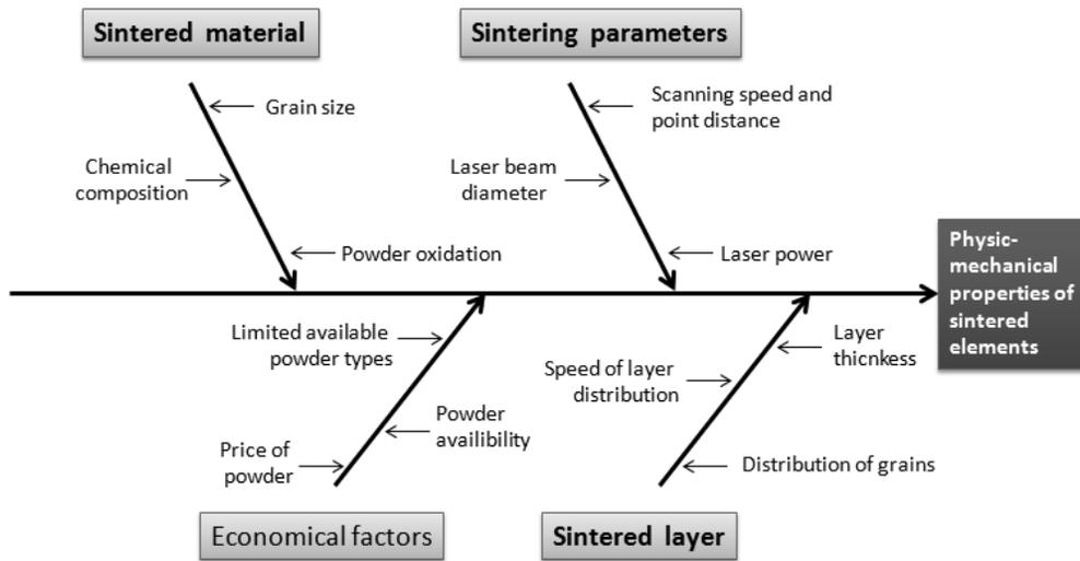
Fig. 5. Factors influencing physic-mechanical properties of SLS manufactured elements
