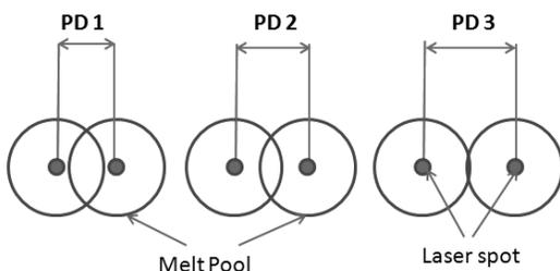
Fig. 7c. Schematic illustration of Point Distance parameter
