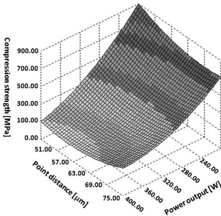
Fig. 10. Compression strength vs Point distance and Laser Power with constant exposure time and scan speed (ET = 92 μs, SP = 87 mm/s)
