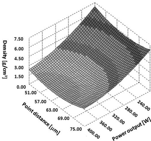
Fig. 11. Density vs Point distance and Laser Power with constant exposure time and scan speed (ET = 100 μs, SP = 84.5 mm/s)
