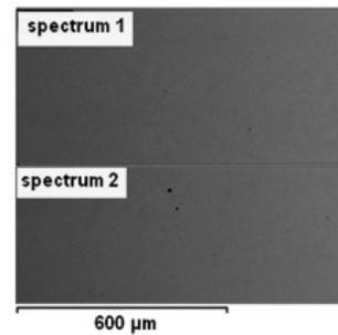
Fig. 12. SEM photo of samples microstructure with visible small pores of diameter not exceeding 10 μm
