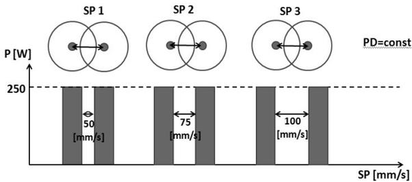
Fig. 7a. Schematic illustration of Exposure Time parameter
