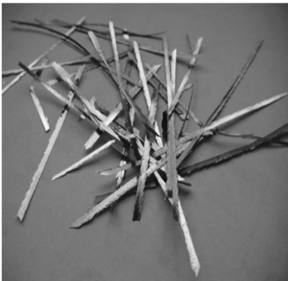
Fig. 2. The research material in Fe_{73}Ni_5Y_3B_{19} ribbon
