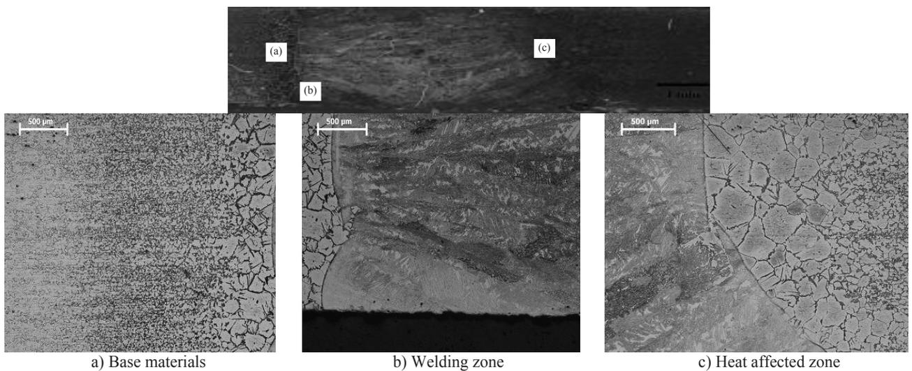
Fig. 2. The macro and the microstructure of a specimen welded with MIG
