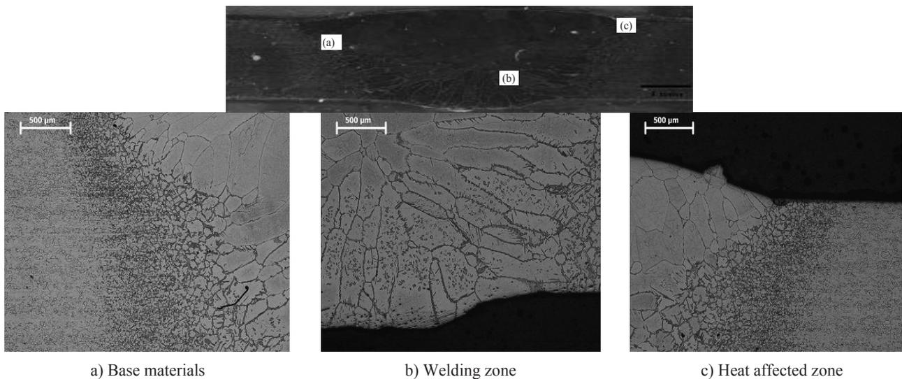
Fig. 1. The macro and the microstructure of a specimen welded with TIG
