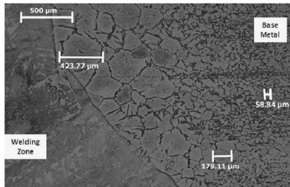
Fig. 3. The microstructure of grain sizes of the TIG (a) and MIG (b) welded specimens
