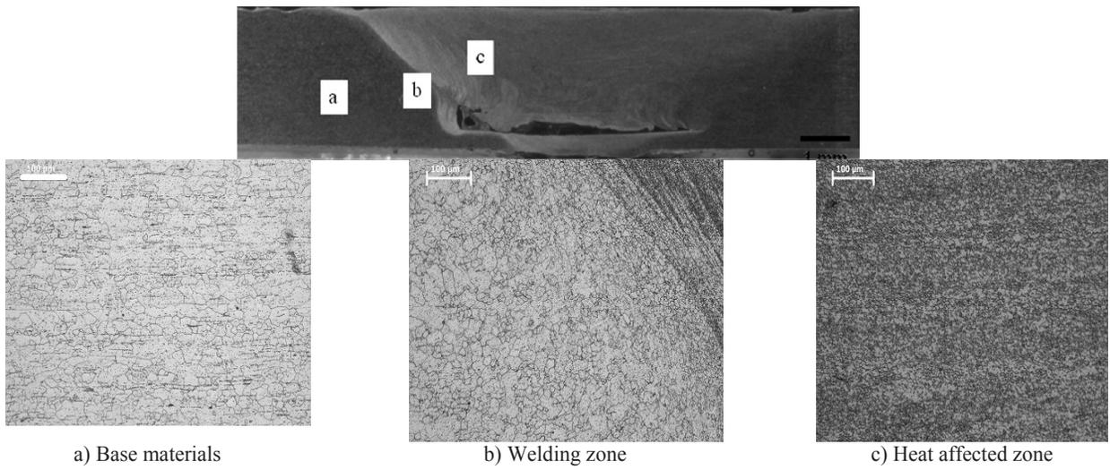
Fig. 5. The macro and the microstructure of a specimen with friction stir welded
