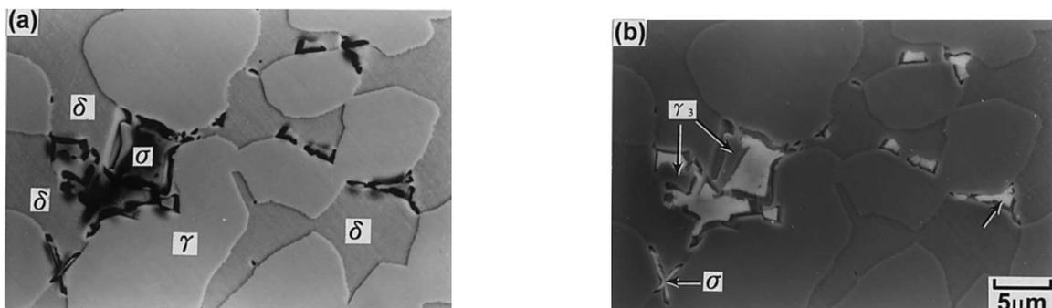
Fig. 4. Scanning electron micrographs showing  $\sigma$  phase located at the  $\delta/\gamma$ -interface, (a) SE and (b) BS images [27]
