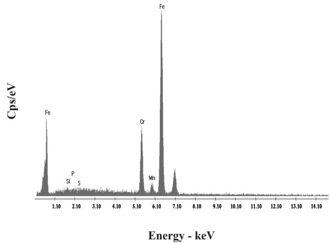
Fig. 7. The SEM results and EDX analysis of uncertain matrix structure in friction stir welded samples
