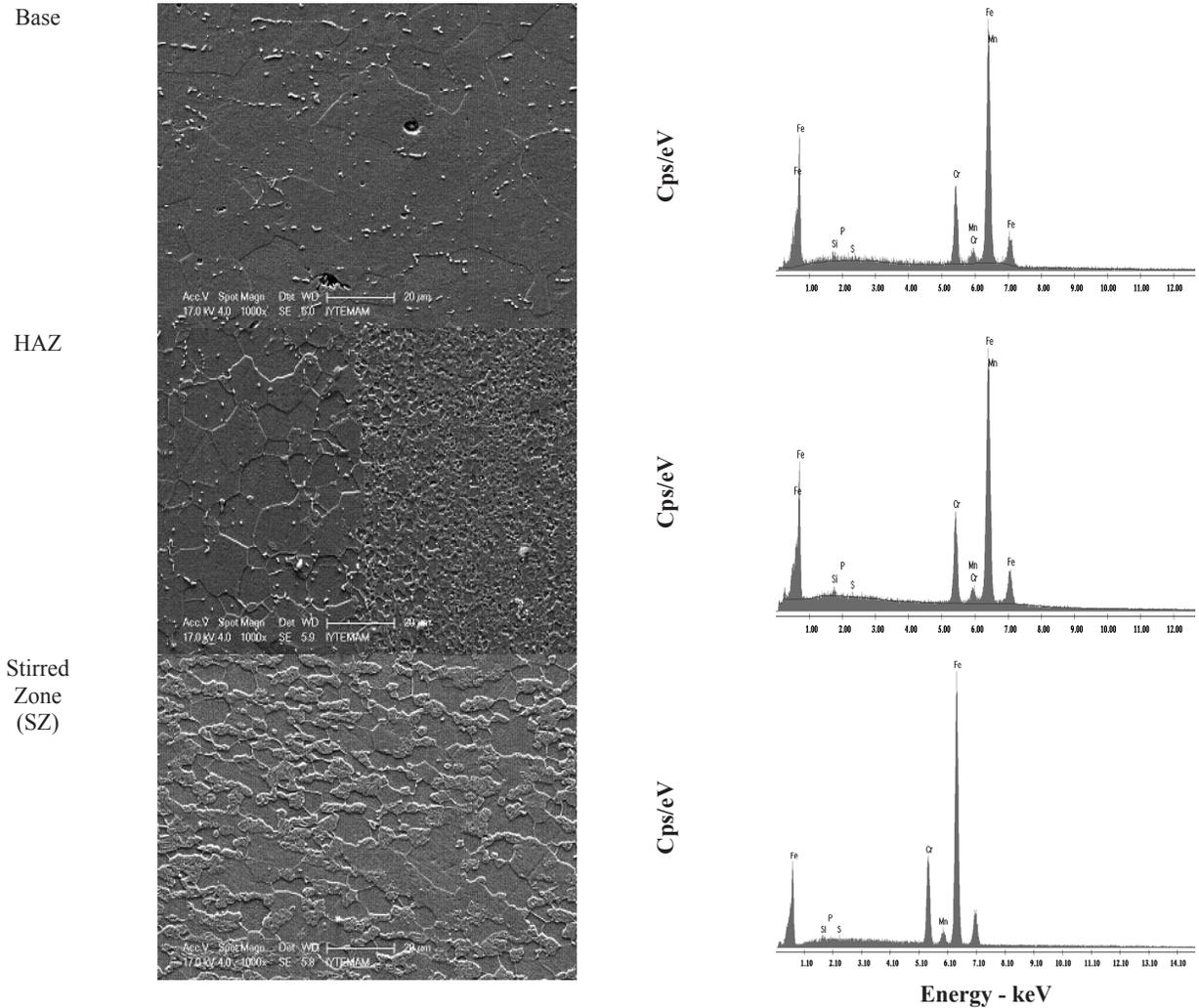
Fig. 6. The EDX analysis of base metal, HAZ, and SZ in friction stir welded samples
