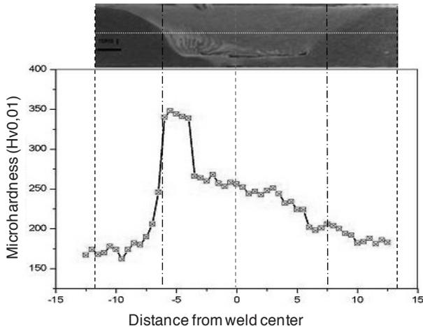
Fig. 8. Micro hardness distributions of friction stir welded sample
