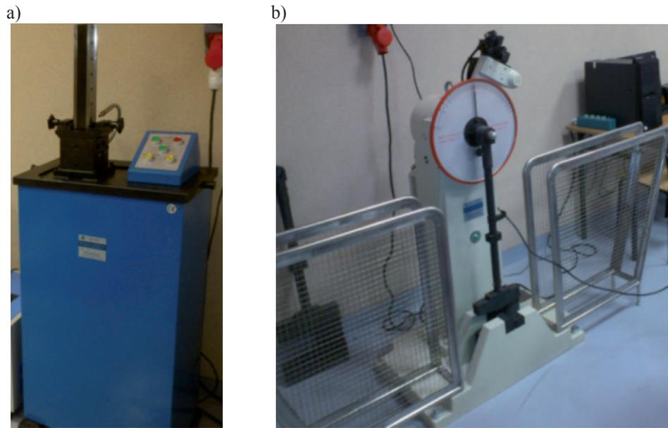
Fig. 2. The devices used during tests a) notches cutter UV L71-UV, b) Charpy impact on the hammer JB-W300A
