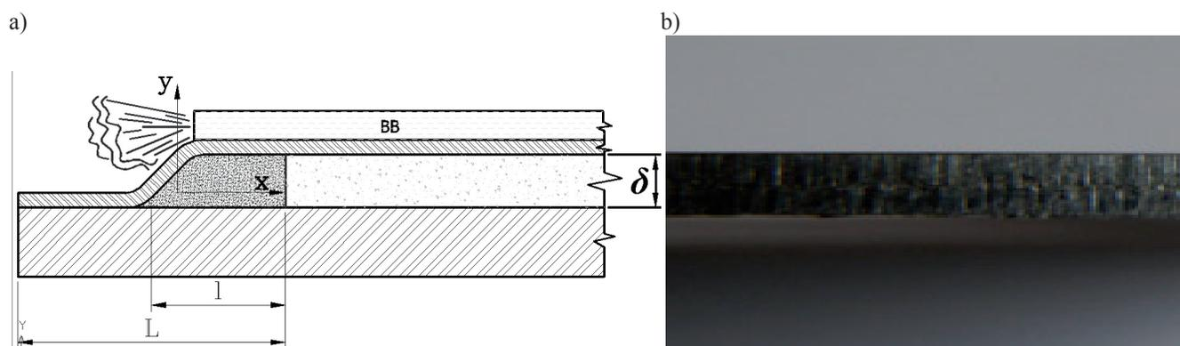
Fig. 1. Scheme of explosive welding (a) and sample of biematlic plate (b) obtained with such technology
