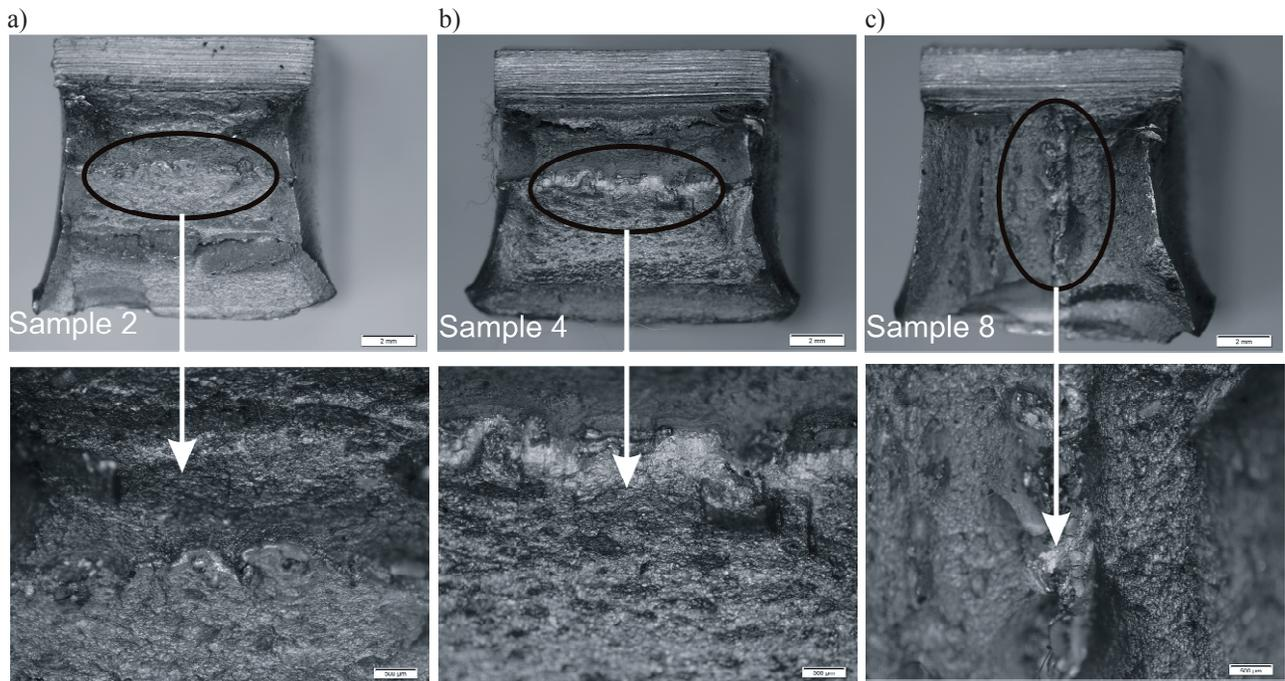
Fig. 4. The breaking area of samples, a) notch cut from the steel PN355NH a1, b) notch cut from the steel X6CrNiMoTi17-12-2 a2, c) notch cut across the height of the bimetal sample a3
