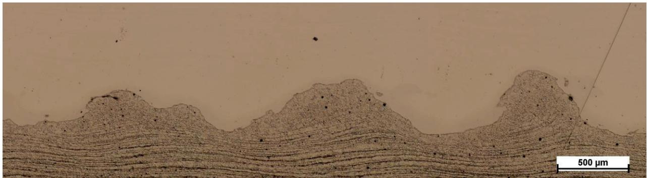
Fig. 3. Photomicrograph of the merging area of the analyzed bimetal. Mag. 50x
