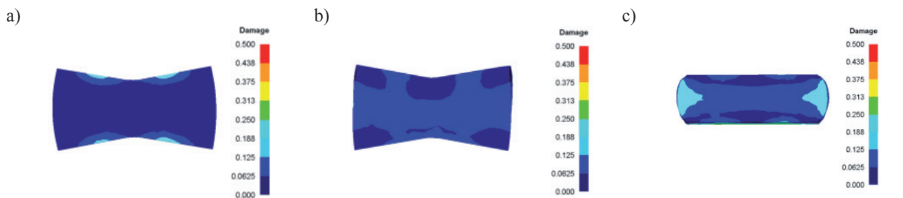
Fig. 4. Damage, a) wedge dies; b) step-wedge dies; c) flat step dies
