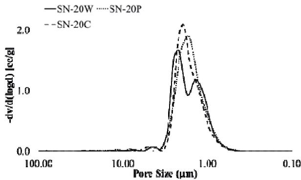
Fig. 3. Pore size distribution of SN-20W, SN-20P and SN-20C
