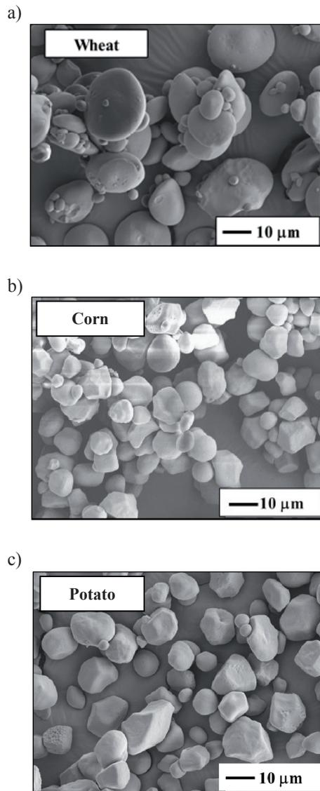
Fig. 1. SEM images of starches a) Wheat, b) Corn and c) Potato
