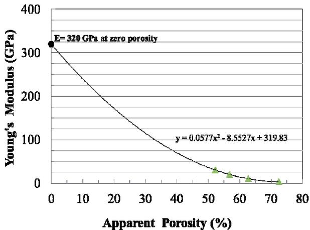
Fig. 4. Young's moduli against apparent porosities of samples produced with wheat starch
