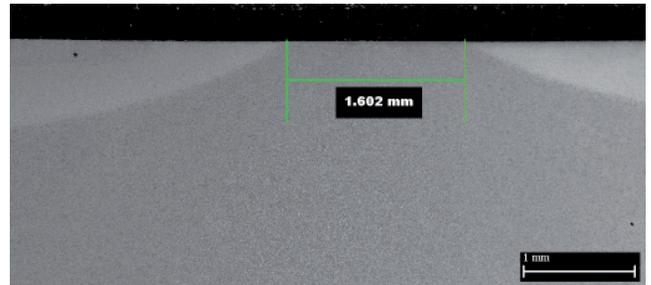
Fig. 4. Hardened material 0 mm overlap (0)
