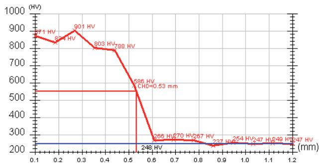
Fig. 12. An example of a measurement record of hardness gradient in the region of the spot overlap axis in a variant of +4
