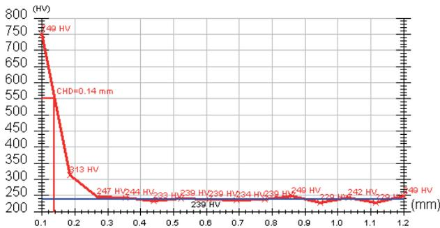
Fig. 7. Example of a measurement record of hardness gradient in the region of the spot overlap axis in the variant of +2
