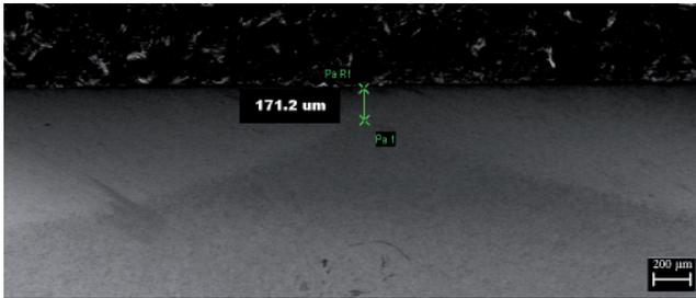
Fig. 6. Hardened material 2 mm overlap (+2)
