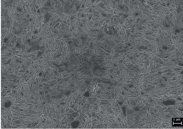
Fig. 11. Hardened material 4 mm overlap (+4) (Point 3 in Fig. 8 – the area tempered when passing the adjacent laser spot)
