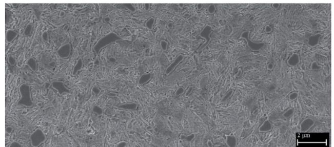
Fig. 5. Hardened material 0 mm overlap (0) (fully hardened area)
