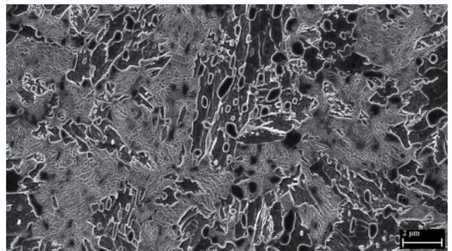
Fig. 9. Hardened material 4 mm overlap (+4) (transition area between the hardened layer and the unhardened parent material – see Point 1 in Fig. 8)
