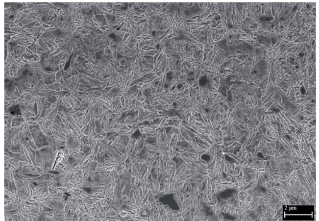
Fig. 10. Hardened material 4 mm overlap (+4) – (the fully hardened area – see Point 2 in Fig. 8)
