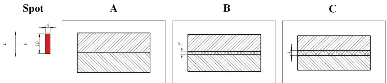
Fig. 1. The schema of three investigated variants of laser spots overlap (A – 0 mm, B – 2mm, C – 4 mm)
