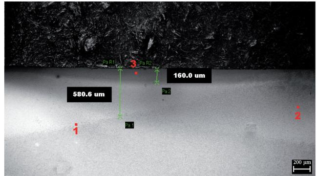
Fig. 8. Hardened material 4 mm overlap (+4)
