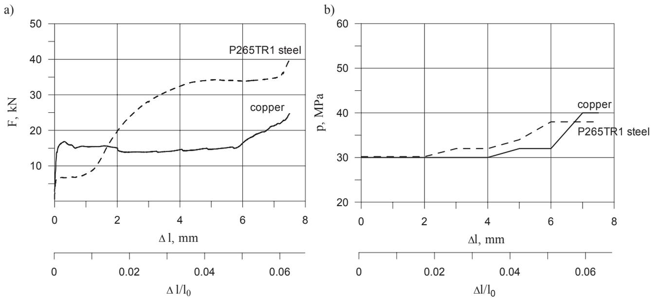
Fig. 3. Force vs. displacement (a) and liquid pressure vs. displacement (b) obtained for hydromechanically bulged axisymmetric components made from copper and P265TR1 steel tubes at ratios  $s_0/D=0.04$ ,  $h/d_1=0.72$  and  $\Delta l/l_0=0.06$
