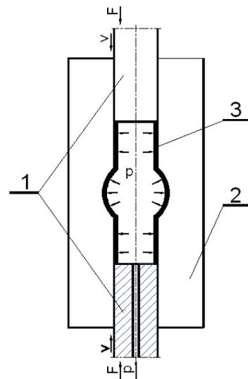
Fig. 1. Hydromechanical bulge forming of axisymmetric component, where: 1 – punches, 2 – die, 3 – component
