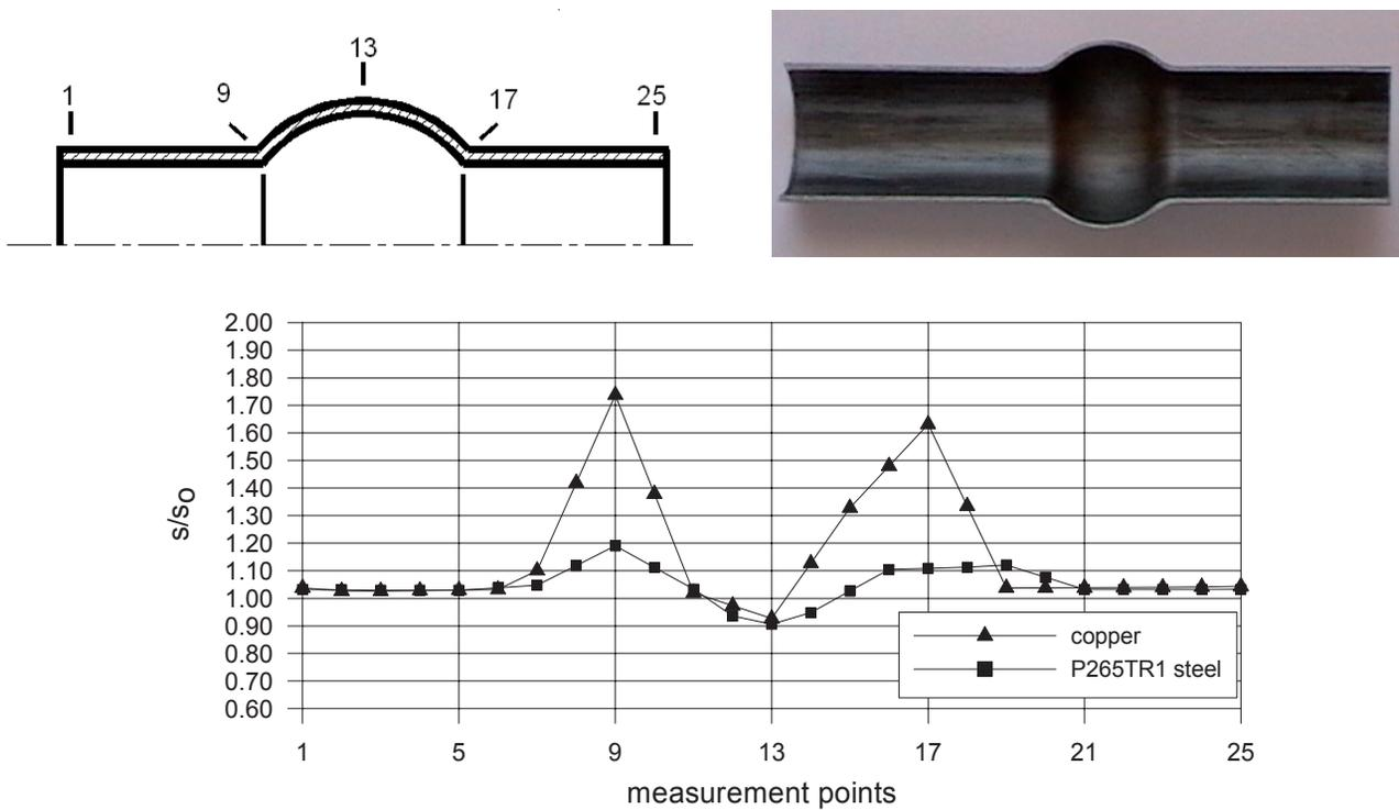
Fig. 4. The wall thickness distribution in longitudinal sections hydromechanically bulged axisymmetric components made from copper and P265TR1 steel tubes at ratios  $s_0/D=0.04$ ,  $h/d_1=0.67$  and  $\Delta l/l_0=0.06$
