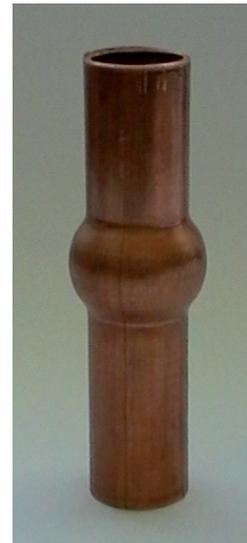
Fig. 2. Hydromechanically bulged axisymmetric components from copper tubes at ratios  $s_0/D=0.04$  and  $\Delta l/l_0=0.062$
