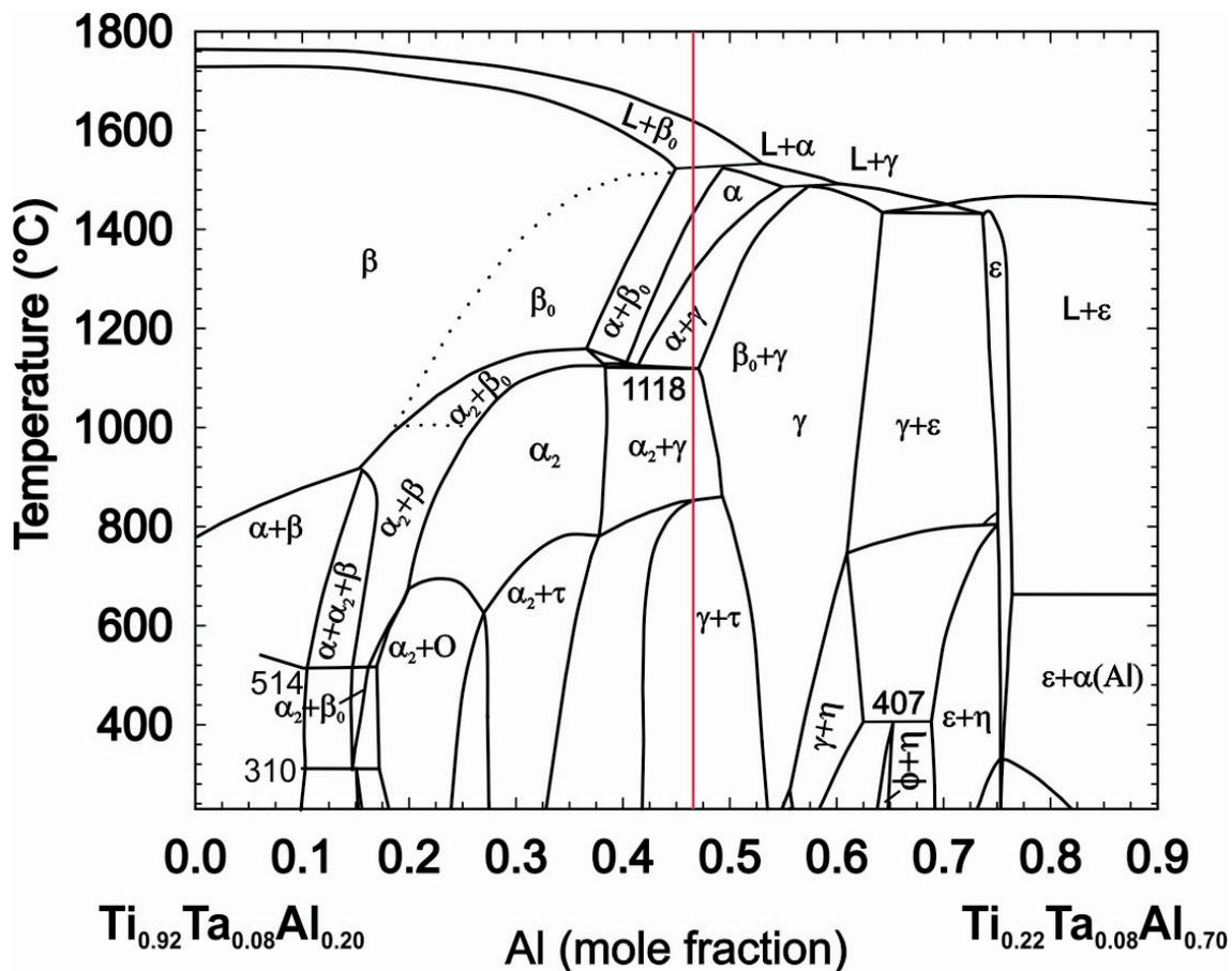
Fig. 1. Calculated isopleth for 8 at.% Ta of the Ti-Al-Ta systems covering the Al composition in the range of 20-70 at.% [5,10]
