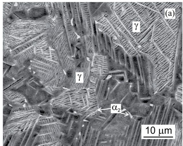
Fig. 2. SEM micrograph showing fine grain structure of as-received Ti-46Al-8Ta (at.%) alloy
