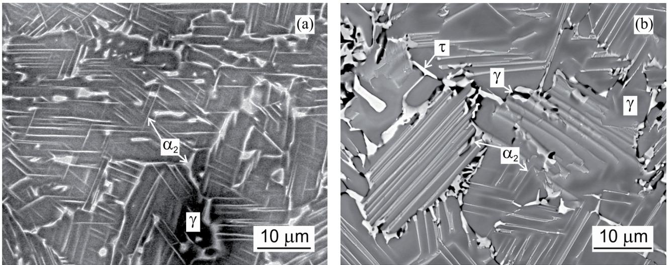
Fig. 3. BSEM micrographs showing the microstructure of Ti-46Al-8Ta (at.%) alloy: (a) as-received alloy composed of  $\alpha_2$  and  $\gamma$  phase, (b) microstructure after annealing at 700°C for 30000 h
