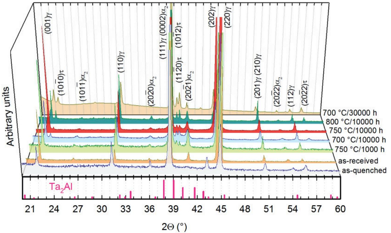
Fig. 4. XRD patterns of the  $\gamma_M$ , as-received and aged Ti-46Al-8Ta (at.%) alloy. The annealing regimes are indicated in the figure
