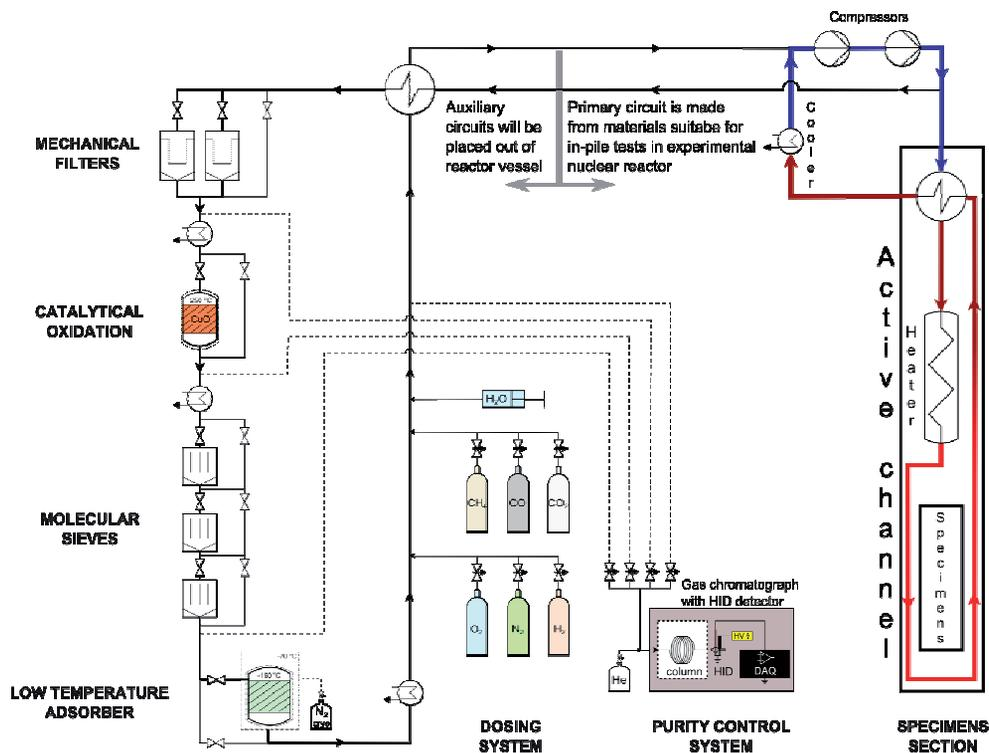
Fig. 1. Experimental helium loop
