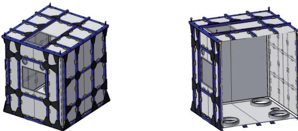
Fig. 6. Steel box with holes for windows, manipulator and entrance for specimens
