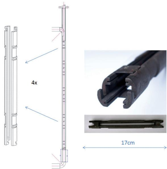
Fig. 3. Holder and test section
