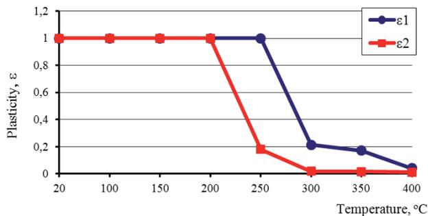
Fig. 4. Influence of annealing temperature of  $\text{Co}_{70.5}\text{Fe}_{2.5}\text{Mn}_{2.5}\text{Mo}_1\text{Si}_9\text{B}_{15}$  metallic glass on the changes of plasticity ( $\varepsilon$ ): 1) for the surface of the ribbon that has not contact with the wheel ( $\varepsilon_1$ ), 2) for the surface of the ribbon adhering to the cooling wheel ( $\varepsilon_2$ )
