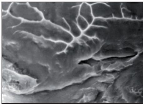
Fig. 3. The structure of the sample fracture in “as quenched” state. “Vein” fracture and a local area with “scaly” morphology
