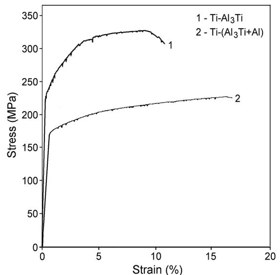
Fig. 1. Tensile curves for the Ti- $\text{Al}_3\text{Ti}$  and Ti-( $\text{Al}_3\text{Ti}$ +Al) composites
