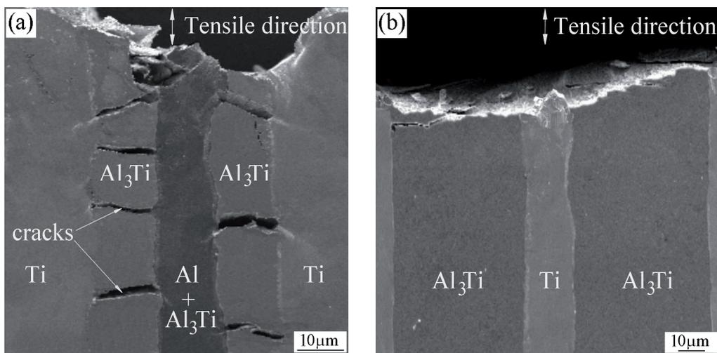
Fig. 2. A cross-section of a fractured Ti-(Al<sub>3</sub>Ti+Al) tensile specimen showing the metals layers bridging many cracks in the aluminide layers (a), and a view of the fracture surface of the Ti50/60 tensile specimen showing brittle fracture of the composite (b)
